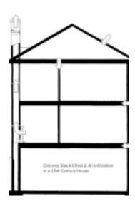
effect of these holes leads to heat loss, condensation in the attic and ice dams. The NegPP is the cumulative effect of leaky basement windows and cracks in the foundation. These holes bring in cold air, leading to dry interior air, cold floors, the chilling of exposed ductwork and the freezing of pipes.
