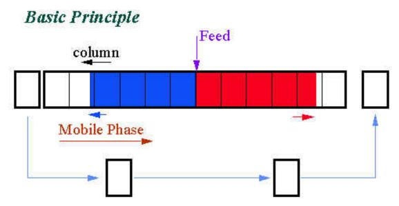
The feed and solvent inlets are now placed between the segments and are moved each time a segment is moved from one end to the other
