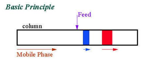
A sample is injected in the centre of a stationary column The two components move at different speeds and are separated
