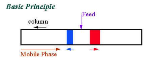
The two solutes now move in different directions relative to a stationary observer. If the column is very long, the bands will continue to separate.
