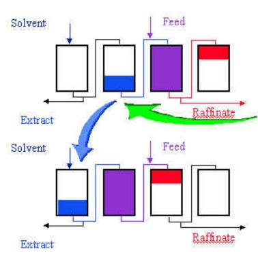
When the mixed band reaches the end of Section 3 its tail has left Section 2 (if the separation has been correctly designed) and only pure product 2 remains in Section 2.
