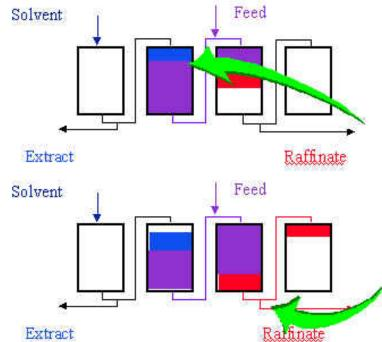
The frontal separation continues, at the same time, the slow moving product starts to separate from the tail of the mixed product band in Section 2
