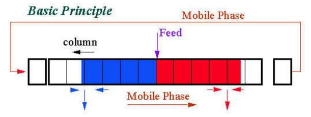
Products are removed by bleeding off a carefully calculated flow at suitable exit points. This changes the velocity of the bands in the column and forces the products to move toward the ports
