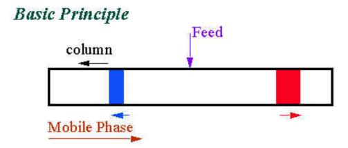
The two solutes now move in different directions relative to a stationary observer. If the column is very long, the bands will continue to separate.
