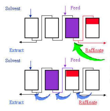
Finally, the mixed product reaches the outlet. To avoid collecting impure material, it is necessary to move the columns 1 position upstream.
