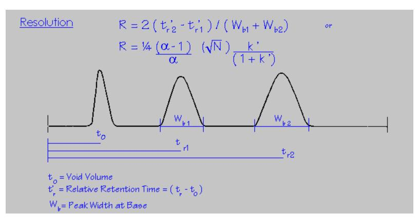
Retention time (tr). The time between injection and the appearance of the peak maximum. The adjusted retention time t'R adjusts for the column void volume. t r' = tr - t0 (or tm).
