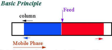
This is clearly a continuous system, but there are problems. It needs an infinite column length and some way to introduce and remove the sample and the products.
