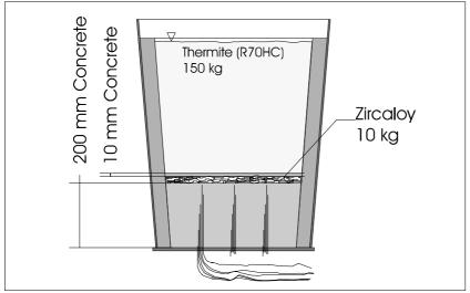
Figure 9: Setup of the KAPOOL 8 container
