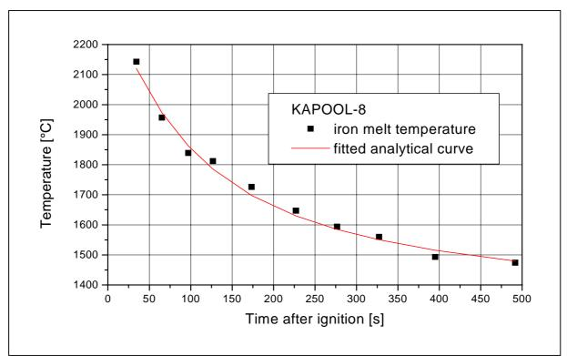
Figure 15: Transient iron melt temperature, included is the fitted analytical curve
