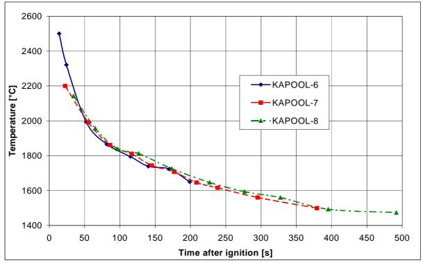
Figure 12: Comparison of the iron pool temperatures in all three KAPOOL tests
