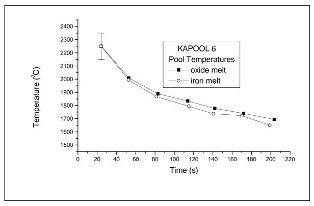
Figure 4: Transient iron- and oxide melt temperatures in KAPOOL 6
