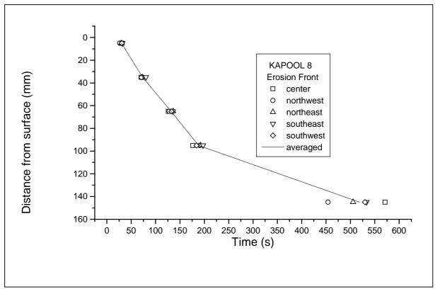
Figure 10: Erosion front in the sacrificial concrete of KAPOOL 8
