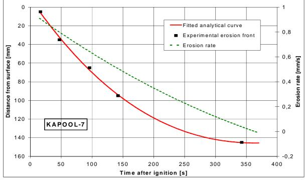
Figure 17: Erosion front with fitted analytical curve and erosion rate
