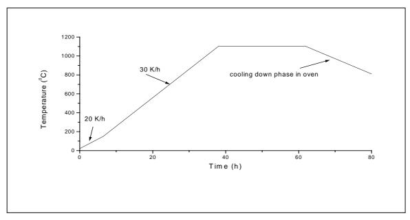
Figure 2: Required temperature treatment of insulating ceramics
