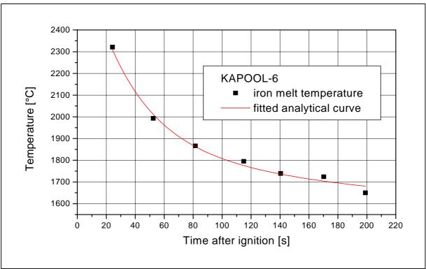
Figure 13: Transient iron melt temperature, included is the fitted analytical curve
