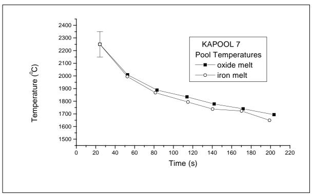
Figure 8: Transient melt temperatures in the iron- and oxide pools of KAPOOL 7
