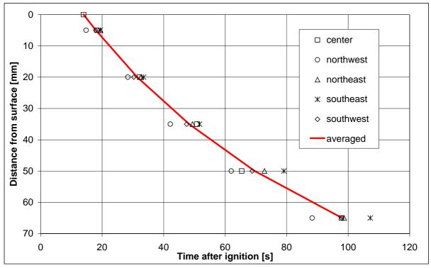
Figure 5: Erosion front in the sacrificial concrete of KAPOOL 6
