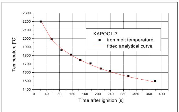
Figure 14: Transient iron melt temperature, included is the fitted analytical curve
