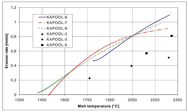
**Figure 19:** Erosion rates for the glass-concrete (KAPOOL 2/3/5) and the sacrificial concrete VM281Q (KAPOOL 6/7/8) as a function of the iron melt temperature
