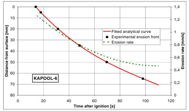
Figure 16: Erosion front with fitted analytical curve and erosion rate
