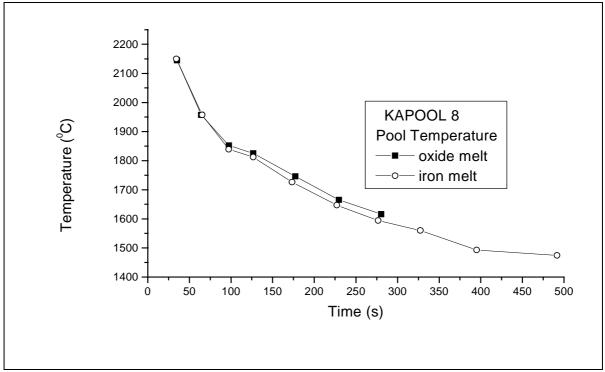
Figure 11: Transient melt temperatures in the iron- and oxide pools of KAPOOL 8
