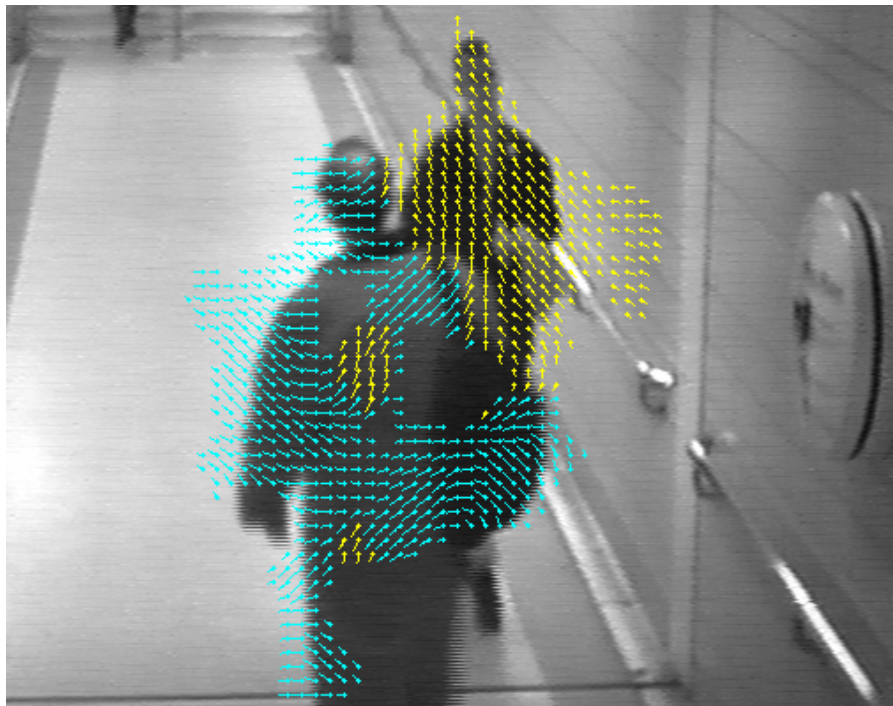
Figure 5: Motion direction detection in a corridor with bad perspective.
