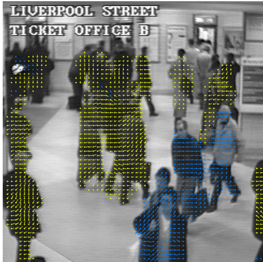
Figure 4: Motion direction detection in underground station's ticket hall with good perspective view.
