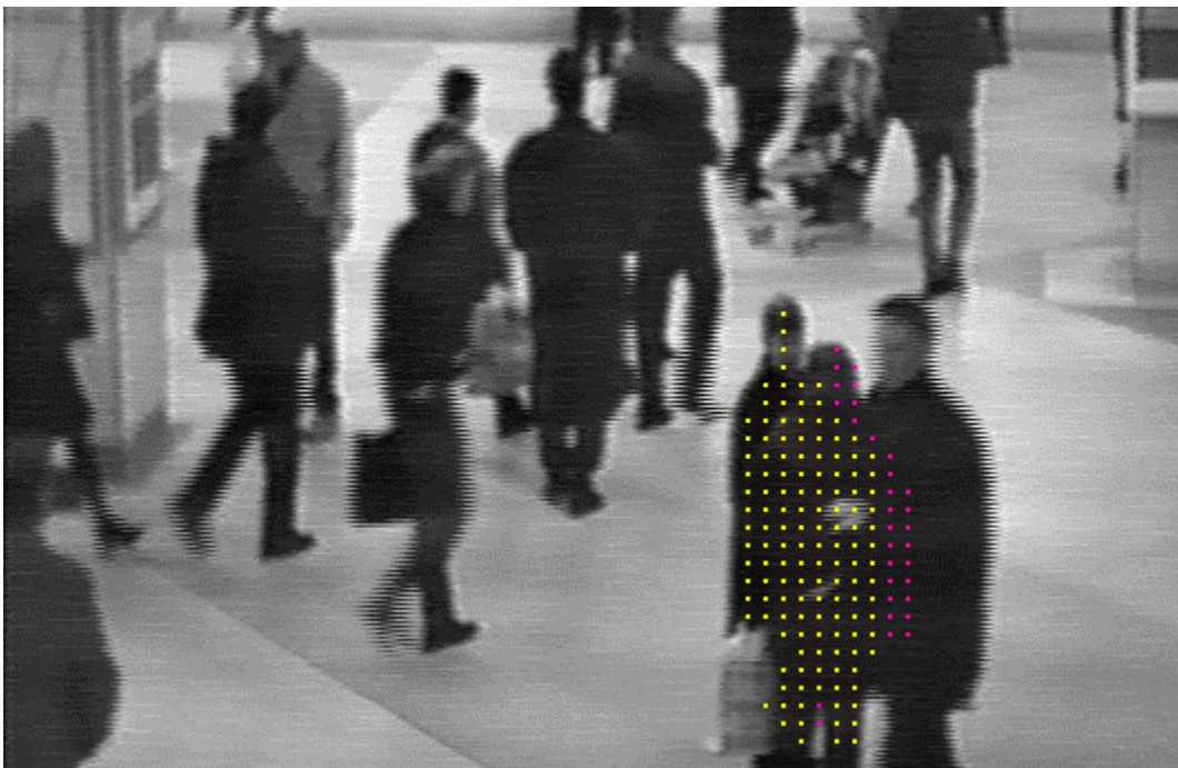
Figure 6: Detection of occluded stationary pedestrians and updating their position.
