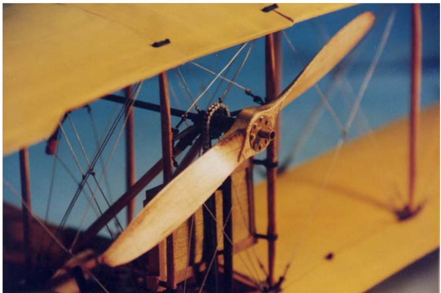
A view of the pusher propeller arrangement. The shaft was chain driven from below. (J. D. Fansler Photo)
