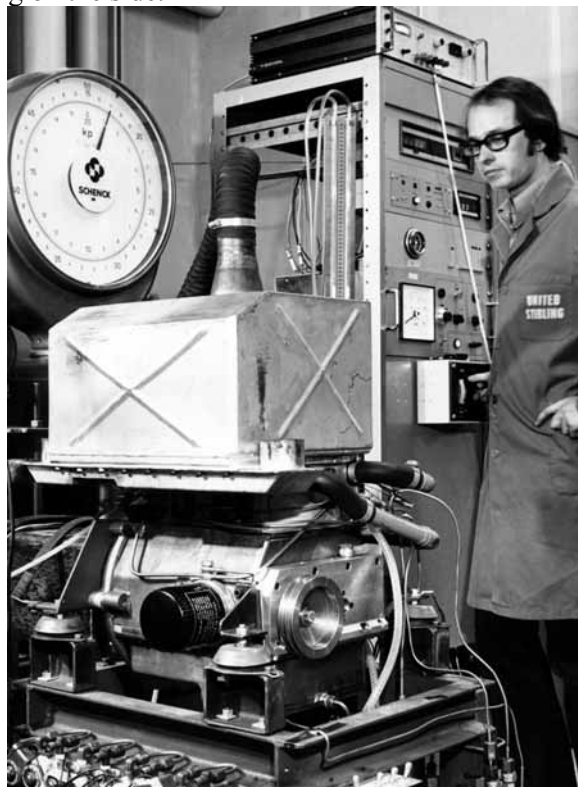
Fig. 3. The V4X1 engine in dynamometer test.
