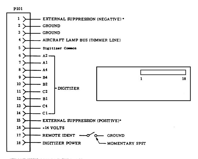
\*TRANSMISSION MAY BE SUPPRESSED BY EITHER: a) GROUNDING PIN 1 OR b) APPLYING A POSITIVE VOLTAGE TO PIN 15
