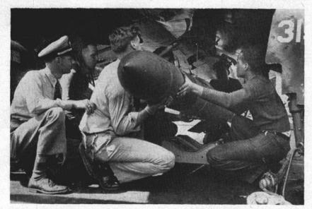
THERE'S nothing tiny about the wallop of this 1000-lb. 'Tiny Tim' rocket being slung under the wing of an F4U Corsair for demonstration in Europe.
