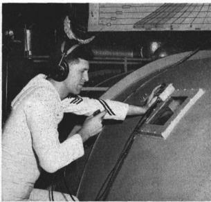
HOSPITAL corpsman checks conditions in oxygen chamber. Right: Inside chamber, men test each other's reactions.
