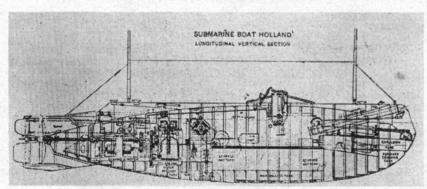
CROSS-SECTION of Holland reveals location of armament. The submarine could be powered by 45-horsepower gasoline engine or an electric motor.
