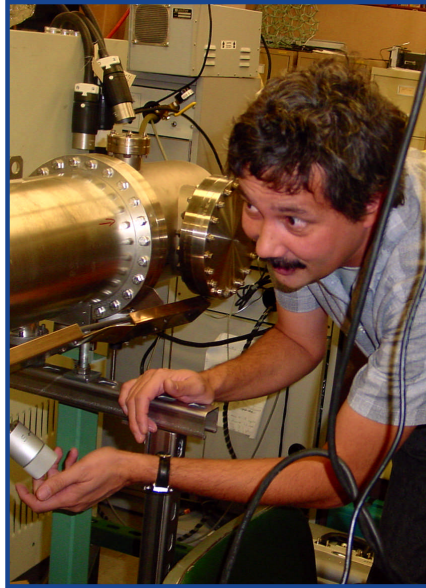
Prof. Idzerda transfers a substrate for magnetic thin film growth under ultrahigh vacuum conditions.
