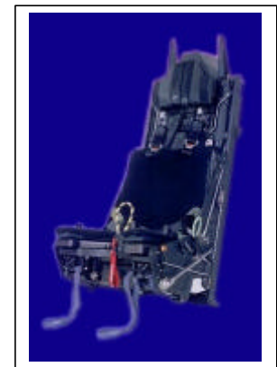
Figure 8.10 Martin Baker Mk 16 L (Courtesy of Martin Baker Aircraft Company Ltd)
