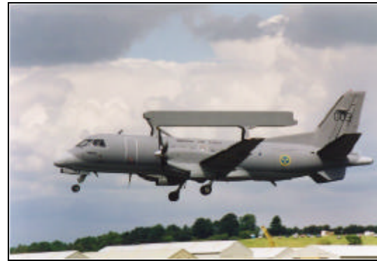
Figure 8.5 Ericsson PS-890 Erieye Radar (Courtesy of the Airborne Early Warning Association. www.aewa.org .)
