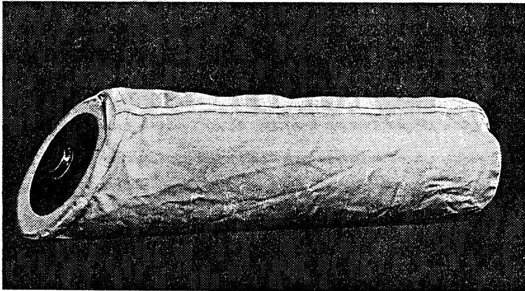
FIGURE 9-10 PARACHUTE EJECTOR BAG
