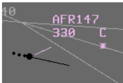
Fig. 5 - 3a : Radar Label - Callsign, Mode C, next sector and * indicating line 4 data present
