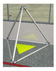
The Goals are three-dimensional tetrahedral shapes, with each face in the form of an equilateral triangle. Each edge of the shape is defined by a six-foot length of 1-1/4" Schedule 40 aluminum pipe (approximately 1.6" OD). The ends of the pipes are attached to "Tetra Connector" to form each apex of the Goal. When properly constructed, the top of the Goal is approximately 5-1/4 feet from the floor.
