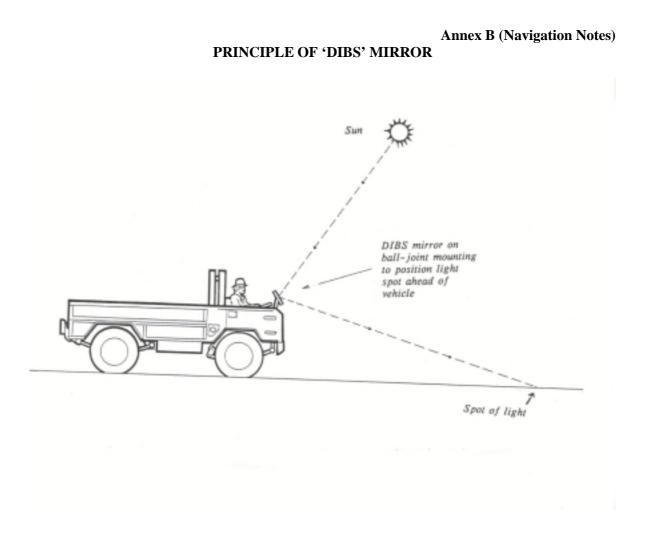
*Optimum mirror to use of DIBS application is about 6in x 8in and must be flat: a convex mirror will not project a light spot.*
