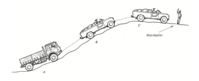
Marshaller first waves vehicle B forward till tow-rope A-B is taut; then he ensures tow-rope B-C is taut. Then, with all three vehicles' engines used and all in the best gear (low range, second gear, in this case in order not to over-torque the loose ground), he drops his arm and on the signal all three drivers let in their clutch. It is essential that all the drivers take their 'go' signal and 'stop' instructions from one man – the marshaller.
