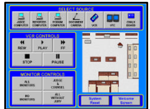
Control System Main Screen – Boston, MA
