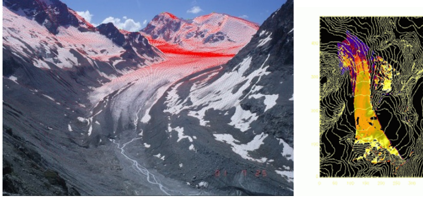
Fig. 4. Example of the technique used to estimate the ratio of snow cover and the spatial distribution of albedo, in this case applied to an Alpine glacier, Haut Glacier d'Arolla. On the left photograph the perspective projection of the DEM appears as red dots, and from these, the georeferenced map of reflectance values on the right image is produced.
