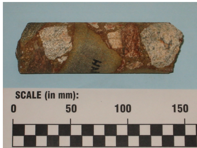
Figure 4: A core sample of the conglomerate from Harvey Dam, indicating clasts of granite and dolerite in a sandstone matrix.
