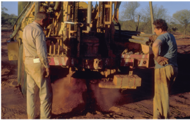
Using a Mayhew to drill a shothole with compressed air at Giles Junction, west of Emu, for Namco International Geophysics Ltd in 1962. (Photo T6491)
