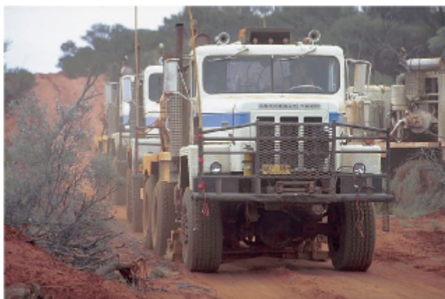
Geosystems Pty Ltd Vibroseis trucks operating on the Officer Basin seismic survey in August 1993. (Photo 41474)
