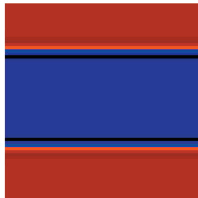
Figure 10. Real part of the total A monomer volume fraction field for a symmetric, ternary blend of A homopolymer, B homopolymer, and symmetric AB diblock copolymer. The homopolymers are mixed in equal proportions and have equal degrees of polymerization, N/2 , half of the diblock copolymer degree of polymerization N . Relevant parameters are \chi N = 9.5 , L = 48 , and \Delta x = 0.75 . Panels a and c denote saddle point configurations with total homopolymer volume fractions of \phi_H = 0.45 and \phi_H = 0.8 , respectively. Panel b shows an instantaneous configuration after a 200 000 time step FTFS simulation (with CL sampling and C = 100 ) of a blend with an intermediate composition, \phi_H = 0.65 , very close to the Lifshitz composition, (\phi_H)_L = 2/3 .
