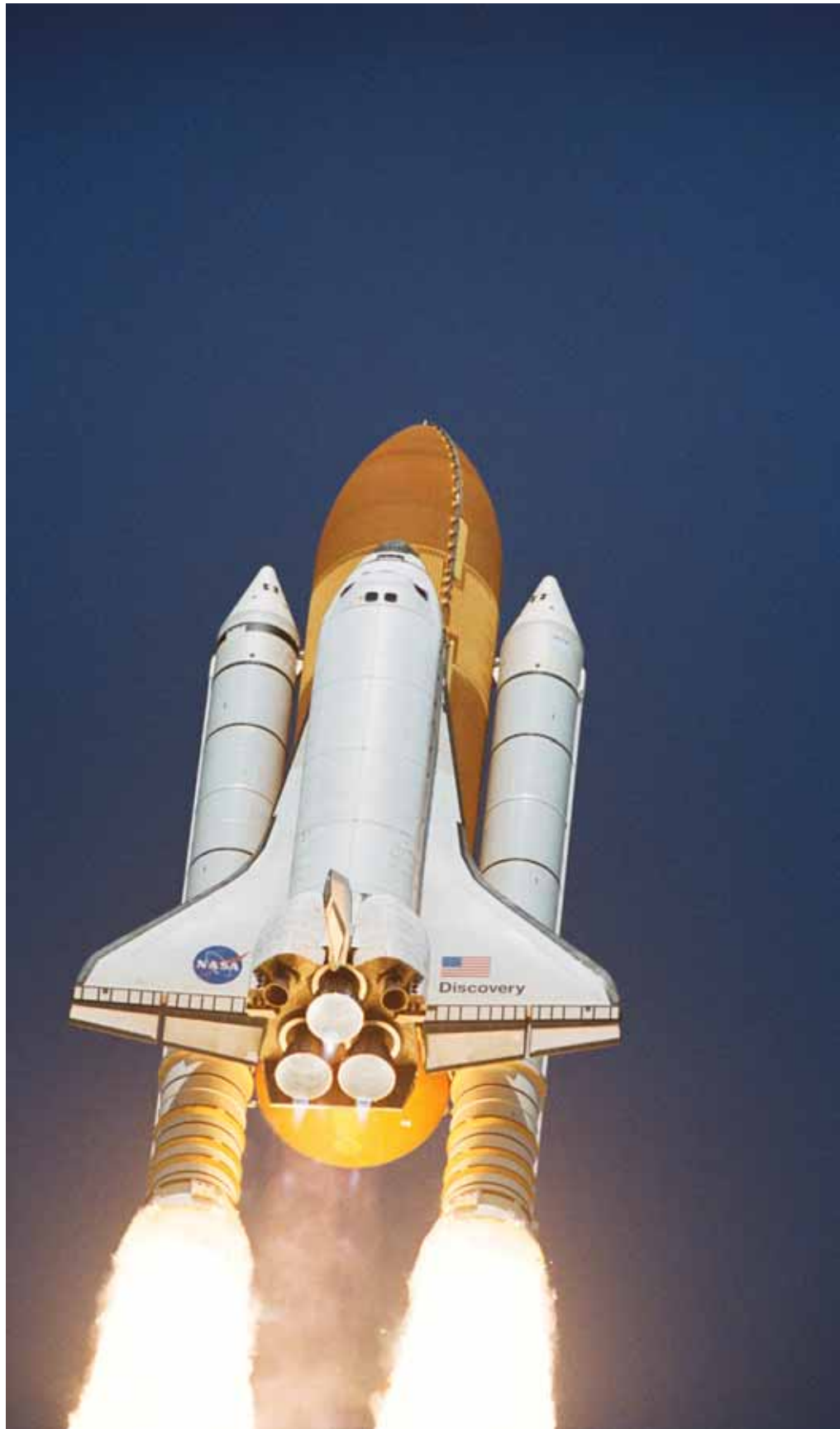
Discovery during ascent with both Solid Rocket Boosters and all three Space Shuttle Main Engines at full throttle.
