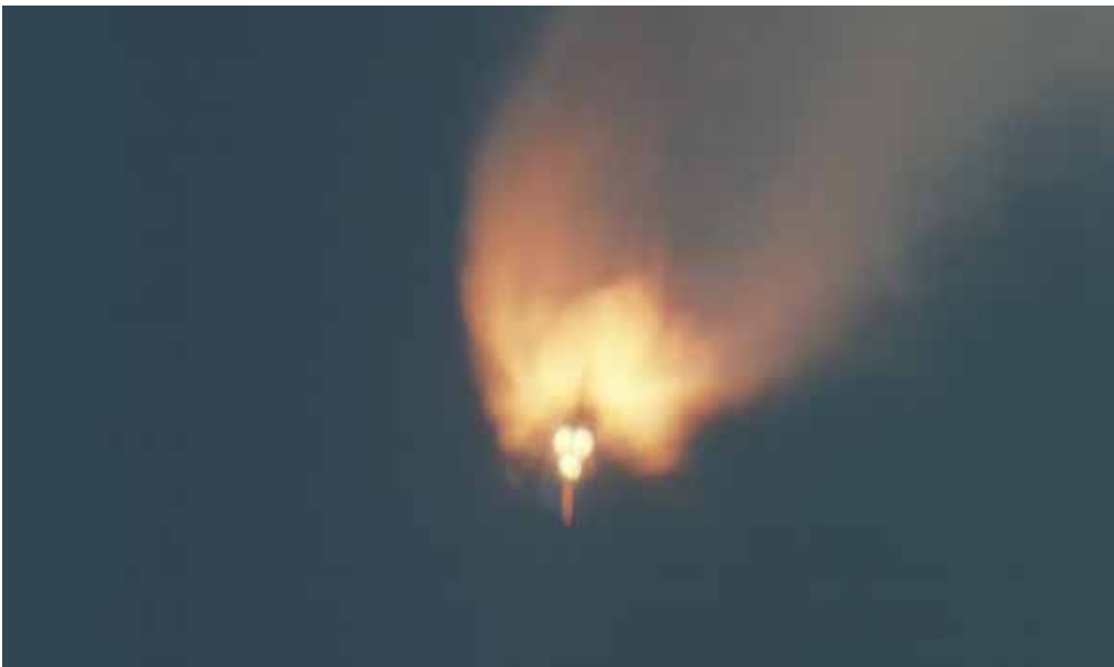
Long-range tracking camera (E-207) photo of STS-95 in October 1998 at SRB separation shows the resolution limitations of ground tracking.
