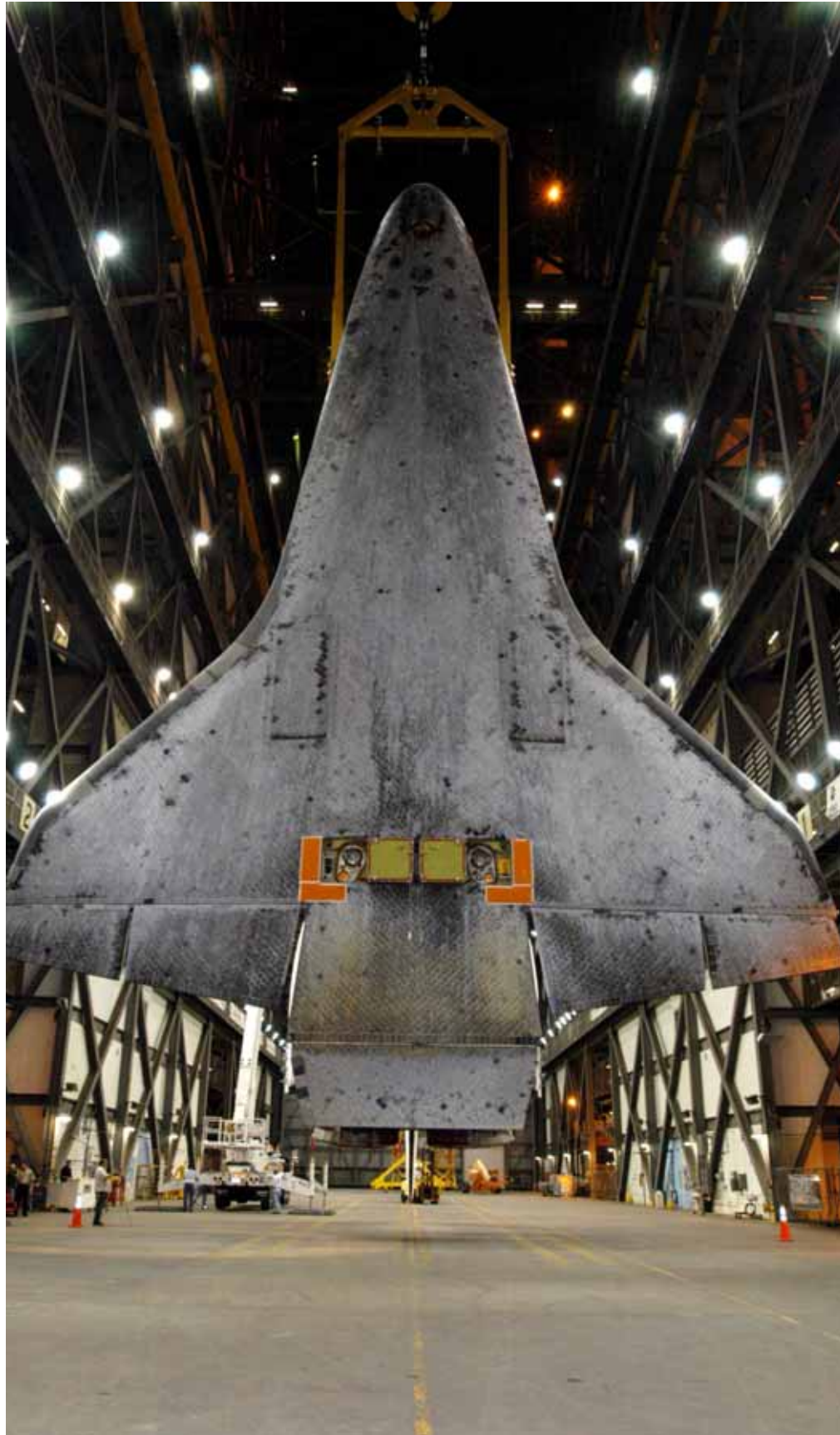
Discovery hangs in the transfer aisle of the Vehicle Assembly Building at the Kennedy Space Center. The two green squares are the undersides of the umbilical well doors; after the External Tank separates, these doors close over the areas just outboard of them.
