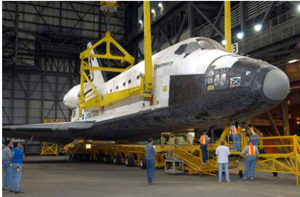
Discovery in the Vehicle Assembly Building transfer aisle, ready to be lifted to the vertical position in preparation for mating with the External Tank and Solid Rocket Boosters.
