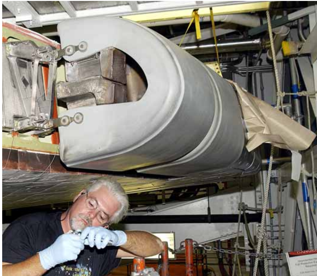
Billy Witt, a midbody shop mechanic with United Space Alliance, checks a part used for installation of a reinforced carbon-carbon panel to the leading edge of the wing of an Orbiter. Note the insulation between the RCC panel and the wing spar.
