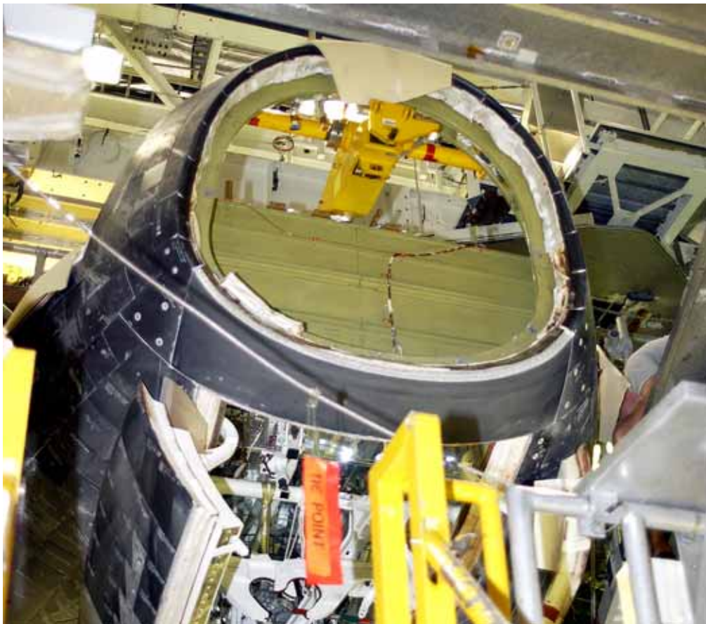
Discovery during early processing for STS-114. The reinforced carbon-carbon nose cap had been removed and returned to the vendor for testing. Note the open nose landing gear door at the bottom left.
