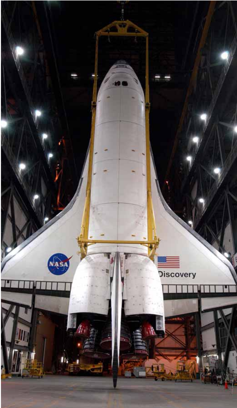
Discovery being lifted to a vertical position in the transfer aisle of the Vehicle Assembly Building at the Kennedy Space Center. After the Orbiter is vertical, it will be lifted into one of the high bays to be mated with a waiting stack of Solid Rocket Boosters and an External Tank.
