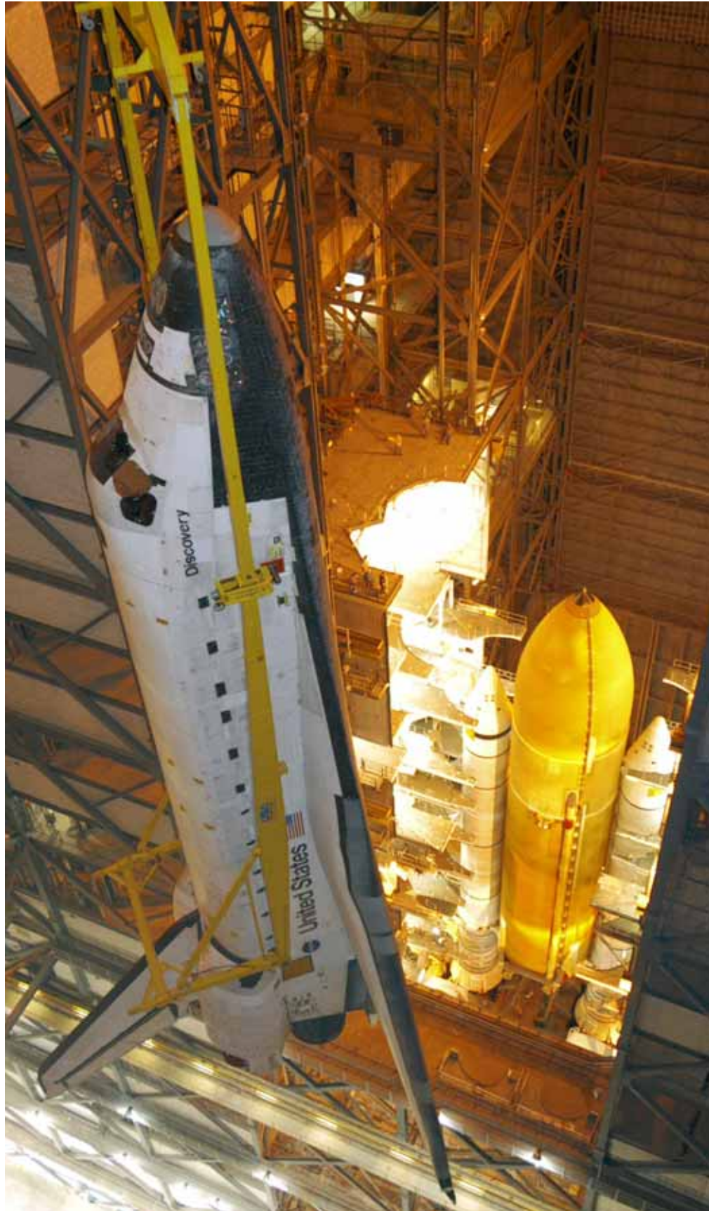
Discovery being lifted onto the stack originally intended for use during STS-114. Anomalies with this External Tank forced the eventually switch to the stack planned for use on STS-121.
