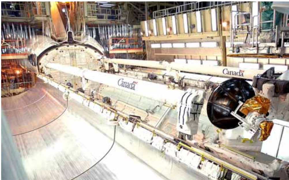
Inside the Orbiter Processing Facility bay 3 at the Kennedy Space Center, Discovery's payload bay doors are ready to be closed. Seen in the center (starboard side) and at right are the new Orbiter Boom Sensor System (OBSS) and the Shuttle Remote Manipulator System (SRMS). The black object in the foreground is the Ku-band antenna.
