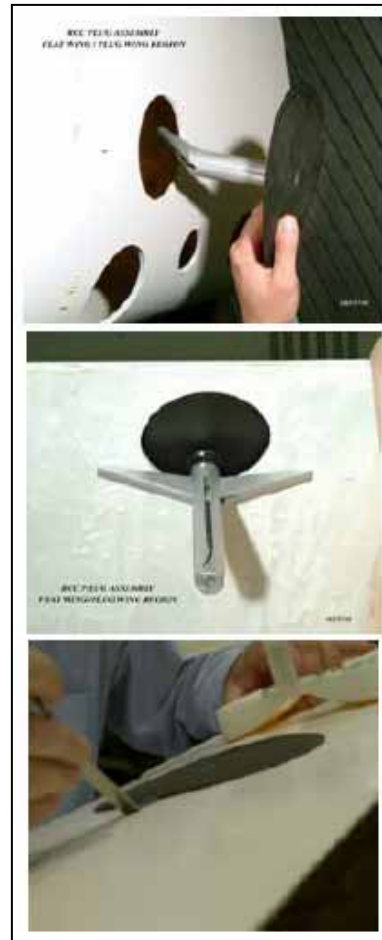
The plug repair starts with either a pre-existing hole in an RCC panel, or with the astronaut drilling a hole. A toggle bolt is inserted through the hole to hold the carbon-silicon carbide cover in place. NOAX is used around the edge as a sealant.
