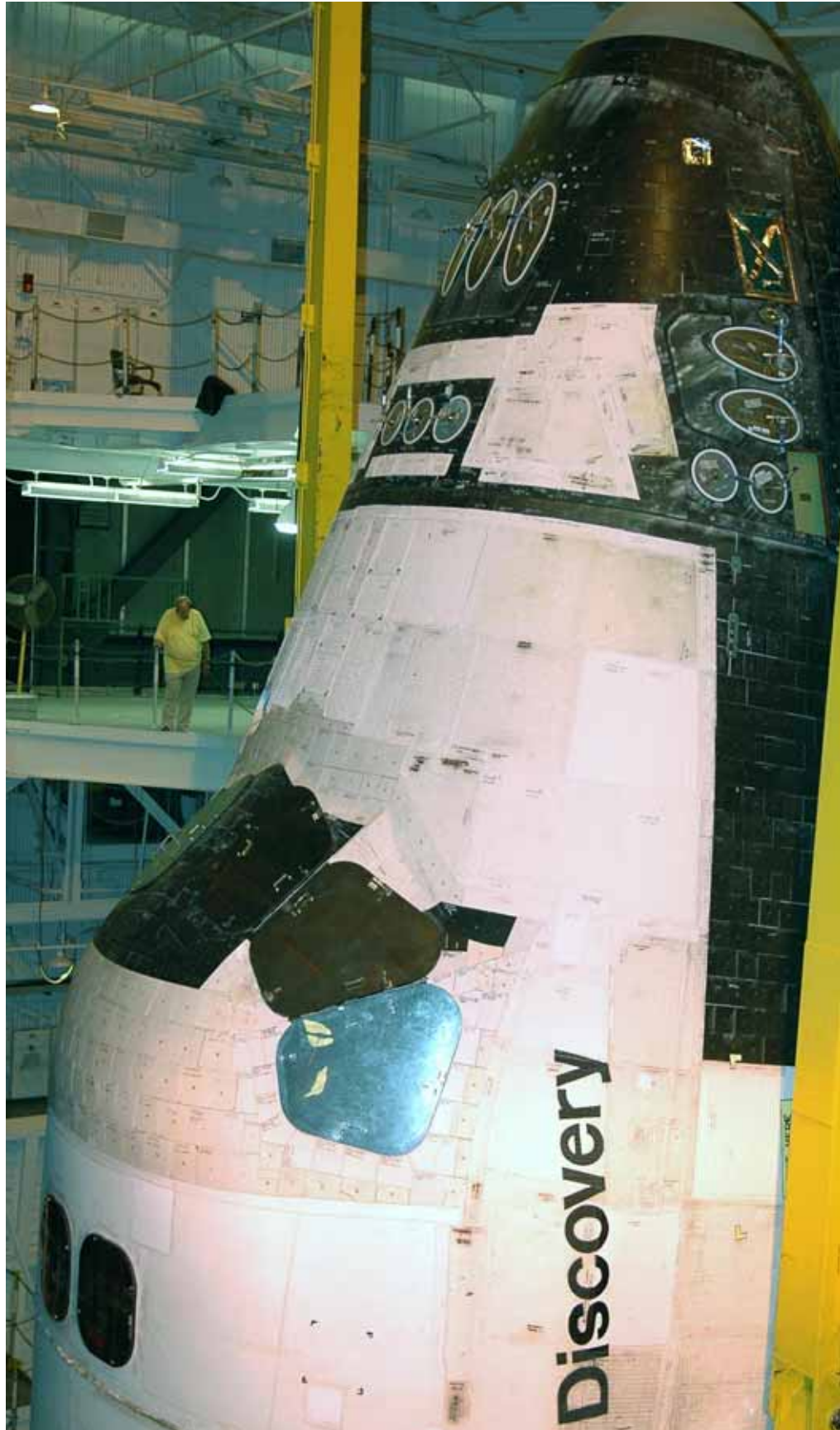
Discovery hangs in the VAB as it is being removed from its original External Tank in the Vehicle Assembly Building at KSC. The Orbiter was later mated with ET-121 prior to the launch of STS-114.
