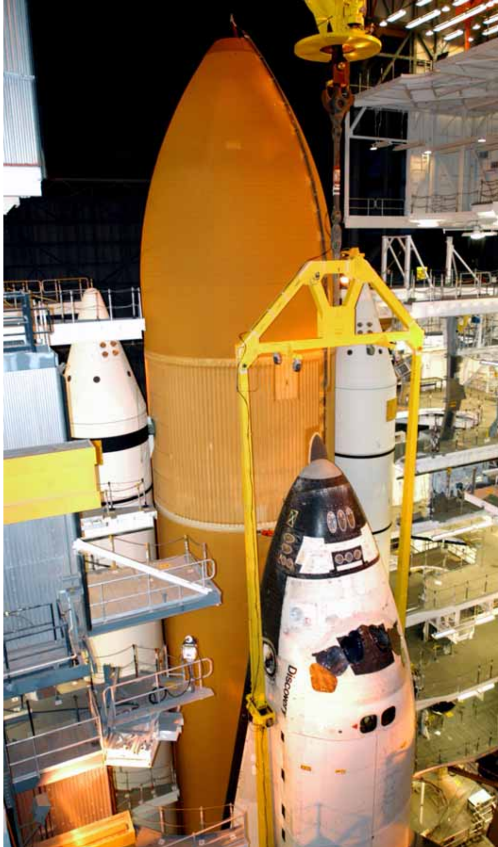
Discovery mated to ET-120 in the Vehicle Assembly Building at the Kennedy Space Center; anomalies with this ET eventually forced the program to switch to ET-121 for STS-114.
