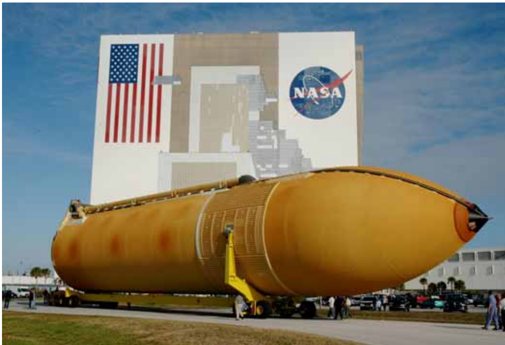
ET-120, the External Tank originally scheduled for use on STS-114, arrives at the Kennedy Space Center. Various anomalies with this tank forced the program to switch to ET-121, the tank originally scheduled for STS-121.
