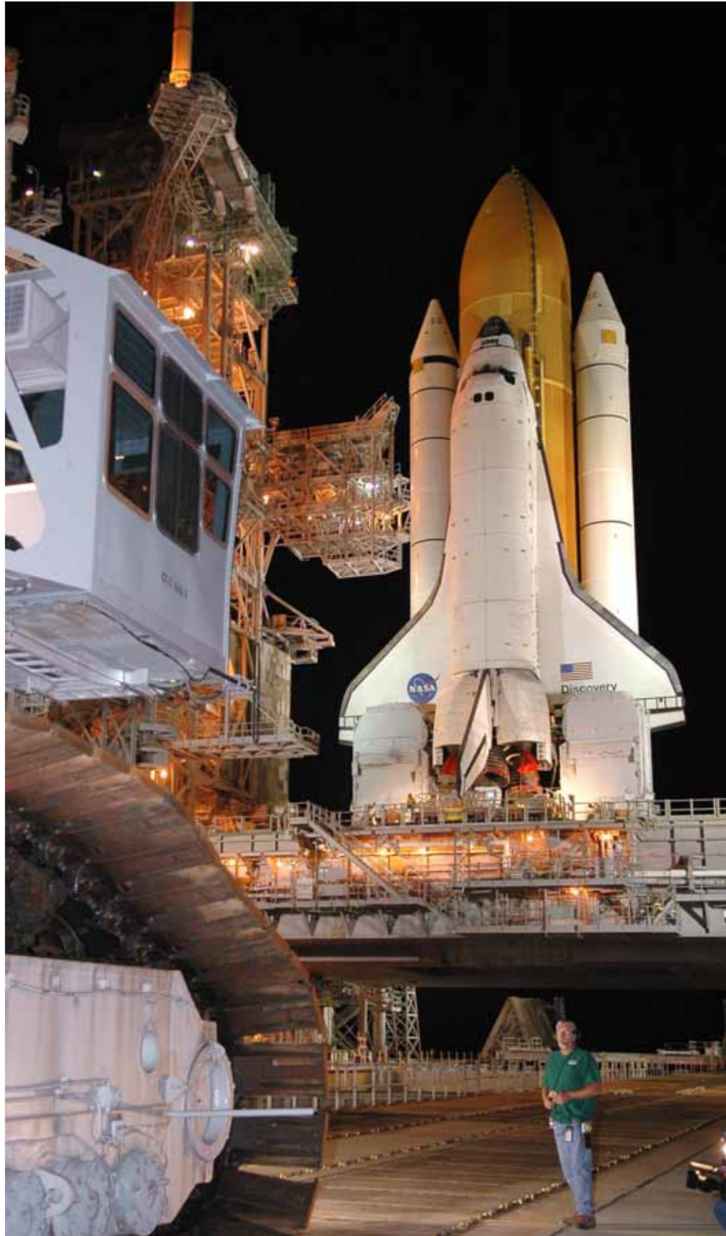
The Crawler-Transporter drives away after delivering Discovery on her Mobile Launch Platform to Launch Complex 39B.
