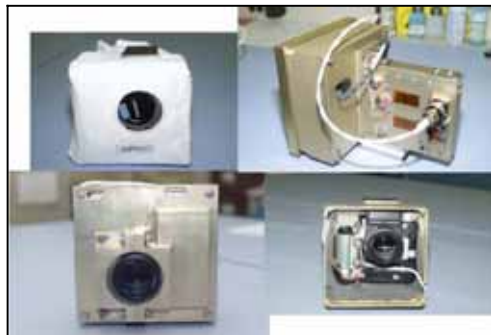
A digital still camera is being carried in the right umbilical well to photograph the External Tank as it separates.
