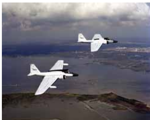
The two NASA high-altitude WB-57F aircraft have been modified with cameras to photograph the Space Shuttle during ascent.
