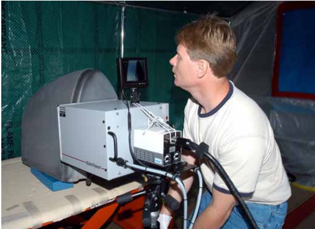
Jim Landy, a specialist with United Space Alliance, examines a wing leading edge carbon-carbon panel using flash thermography. A relatively new procedure at KSC, thermography uses high intensity light to heat areas of the panels. The panels are then immediately scanned with an infrared camera. As the panels cool, any internal flaws are revealed.
