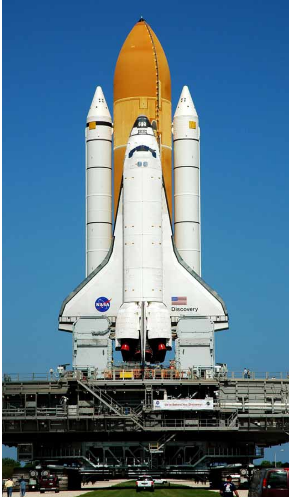
Discovery , atop a Mobile Launcher Platform (MLP), crawls toward Launch Complex 39B on April 6, 2005. The MLP is moved by the Crawler-Transporter underneath. The crawler stands 20 feet high, 131 feet long and 114 feet wide and moves on eight tracks, each containing 57 cleats weighing one ton each. The crawler moves at a maximum speed of approximately 0.8 mile per hour while carrying the 3 million pound Space Shuttle stack. Note the "We're Behind You, Discovery" banner on the MLP.
