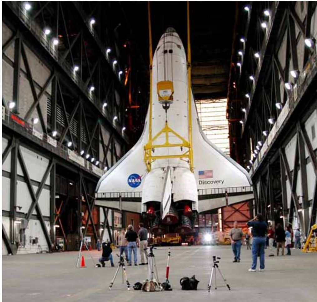
Before a group of photographers, Discovery is hoisted into a vertical position in the transfer aisle of the Vehicle Assembly Building at the Kennedy Space Center. After this the Orbiter was lifted into a High Bay to be mated with a waiting set of Solid Rocket Boosters and an External Tank.
