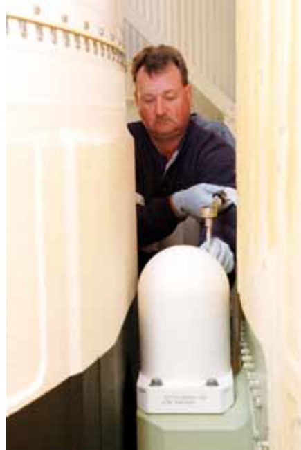
The bolt catchers for ET-120, originally intended for use on STS-114, during their installation at the Kennedy Space Center. The bolt catchers used on ET-121, the tank actually used for STS-114, were identical.
