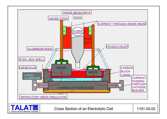
Each cell in a primary smelter produces over 1 tonne of molten aluminium each 24 hours. The operation is continuous for the life of the pot which may well be between 5 and 10 years. With a modern smelter having an annual capacity of 150 to 250 thousand tonnes there will be several hundred pots. The molten metal is syphoned out of the pots and taken to a cast house for further processing.
