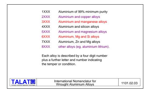
These alloys fall into two main groups (**Figure 1101.02.04**). The work hardening alloys, where strength is related to the amount of 'cold work' applied, by rolling or forming, and heat treatable or precipitation hardening alloys. With the latter strength and other properties are enhanced by heat treatment of various kinds.
