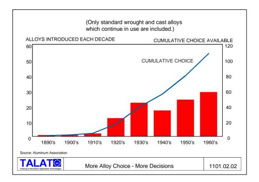
There is an impressive array of commercially available alloys the composition and logic being regulated by agreed international nomenclature. For wrought alloys each is described by a four digit number plus further letter and number indicating the temper or condition of the alloy (see **Figure 1101.02.03**).
