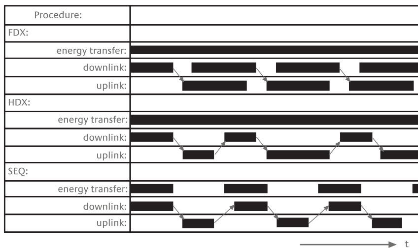
Figure 5-6: Chart showing temporal sequences in full duplex, half duplex and sequential systems. Transmission channel from reader to transponder is called downlink, reverse direction uplink [Source: Fink02]
