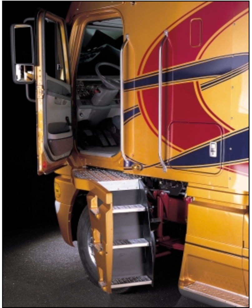
The optional innovative staircase-style steps provide a standard of convenience in cab entry and exit. Electronically controlled, they automatically pivot from under the cab when the door is opened or closed.
