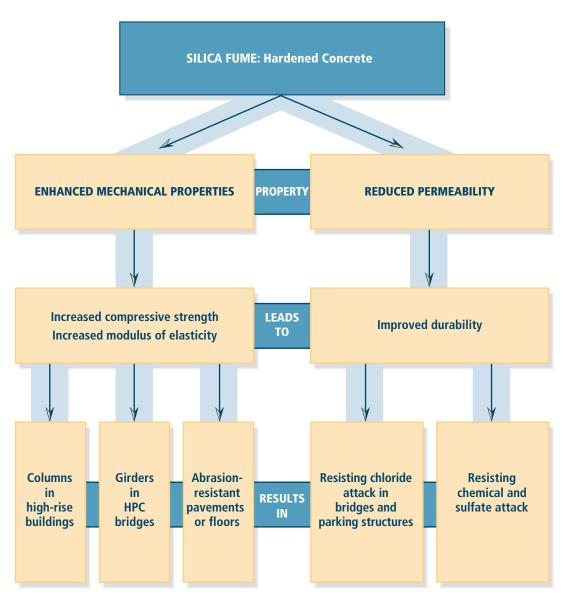
FIGURE 3.5. Effects of silica fume on hardened concrete and how those effects are used in concrete applications.
