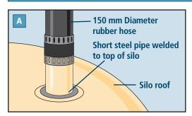
OPTION "A" - Rubber hose connected to steel pipe
