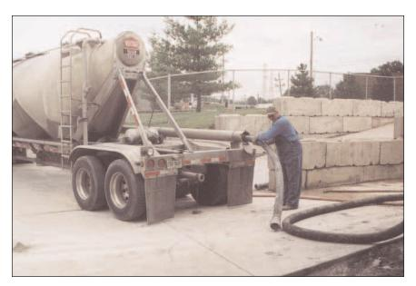
FIGURE 7.5A. Rubber hose used to transfer silica fume from tanker to producer's silo.
