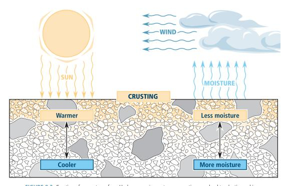
FIGURE 8.2. Crusting of concrete surface. Under some circumstances, crusting may lead to plastic cracking.
