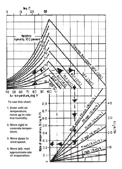
FIGURE 8.1. ACI evaporation estimation chart. Source: ACI 308R, Guide to Curing Concrete.
