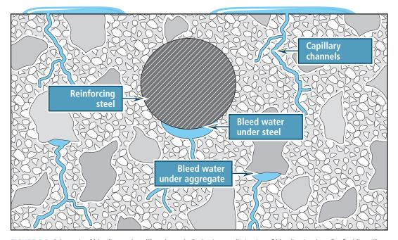
**FIGURE 3.3.** Schematic of bleeding and capillary channels. Reduction or elimination of bleeding is a benefit of adding silica fume to a concrete mixture.
