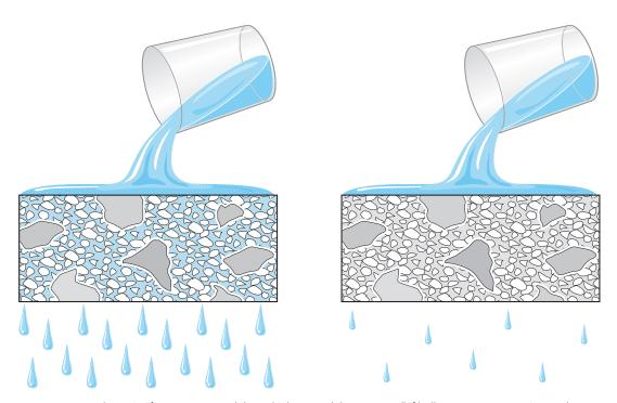
FIGURE 3.11. Schematic of concrete permeability. A high permeability concrete (left) allows water to move into and through the concrete readily. Lowering the w/cm and adding silica fume can reduce permeability to essentially zero. Such a reduction makes it very difficult for water and aggressive chemicals such as chlorides or sulfates to enter the concrete.
