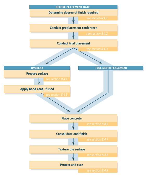
**FIGURE 8.6.** Finishing steps for concrete bridge decks. The steps are described in the text section noted.
