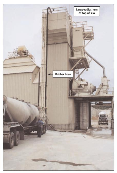
**FIGURE 7.3.** Unloading bulk densified silica fume into a silo. Note rubber hose and large-radius turn at top of silo.
