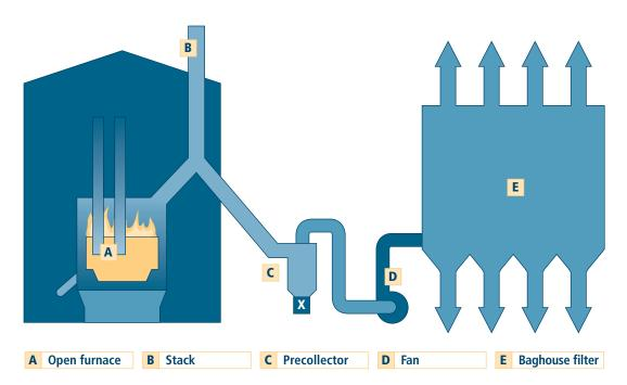
**FIGURE 1.4.** Schematic of a smelter for the production of silicon metal or ferrosilicon alloy. The silica fume is collected in large bags in the baghouse.
