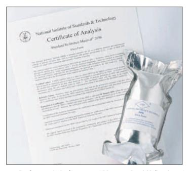
**FIGURE 4.4.** Silica fume Standard Reference Material (SRM 2696) available from the National Institute for Standards and Technology. Check either the Silica Fume Association or NIST web sites, as listed in the text, for instructions on how to order this material.
