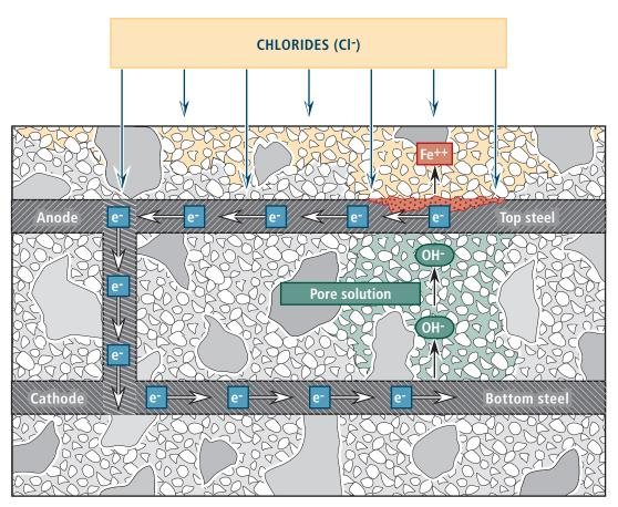
**FIGURE 3.12.** Schematic of corrosion in reinforced concrete. At the anode chloride ions interact with iron to produce Fe++ ions. The electrons released flow through the reinforcing steel to the cathode. The electrical path is completed by OH<sup>—</sup> ions flowing through the pore solution (electrolyte). In some cases the anode and cathode may both be on the same bar. By reducing the permeability of the concrete, silica fume delays the chlorides reaching the steel.
