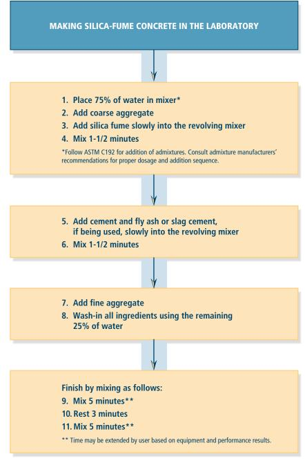
FIGURE 6.2. Recommendations for making silica-fume concrete in a laboratory mixer.
