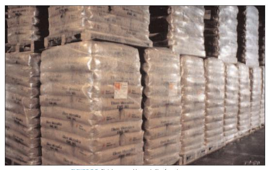
FIGURE 7.7. Shrink-wrapped bagged silica fume in storage.
