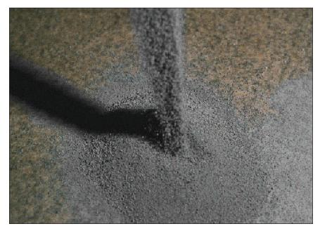
**FIGURE 5.1.**Densified silica fume.
