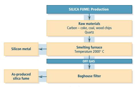
FIGURE 1.3. Schematic of silica fume production.
