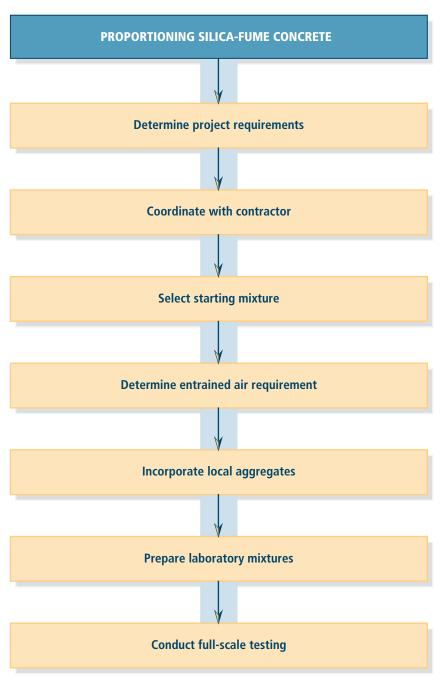
**FIGURE 6.1.** Steps in proportioning silica-fume concrete. Each of these steps is discussed in detail in the text.
