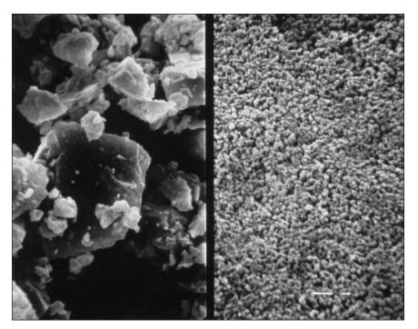
**FIGURE 2.1.** Photomicrograph of portland cement grains (left) and silica-fume particles (right) at the same magnification. The longer white bar in the silica fume side is 1 micrometer long. Note that ACI 234R, *Guide for the Use of Silica Fume in Concrete*, estimates that for a 15 percent silica-fume replacement of cement, there are approximately 2,000,000 particles of silica fume for each grain of portland cement.
