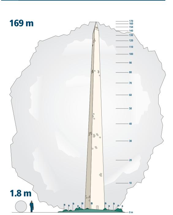
**FIGURE 2.2.** General size comparison of silica-fume particles. If a person (1.8 m) were the size of a silica-fume particle, then a cement grain would be approximately the size of the Washington Monument (169 m).
