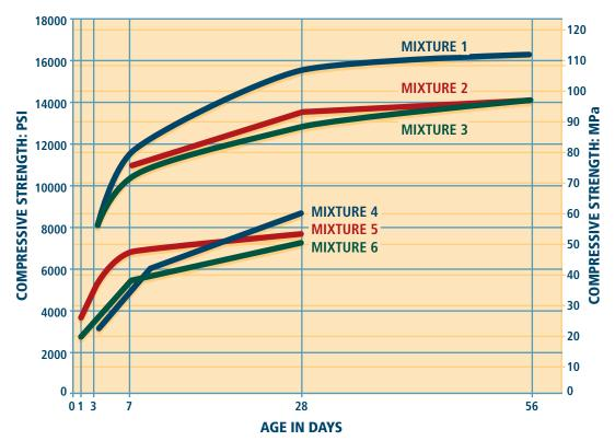
**FIGURE 3.6.** Strength development of several concrete mixtures containing silica fume. Details for the mixtures are provided in the table below.
