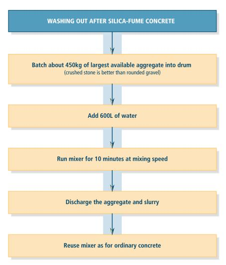
**FIGURE 7.2.** Recommendations for washing out truck mixers after silica-fume concrete. Based upon the NRMCA *Truck Mixer Driver's Manual* (1999).
