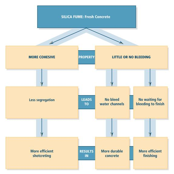
FIGURE 3.1. Effects of silica fume on fresh concrete and how those effects improve constructability and the final concrete.
