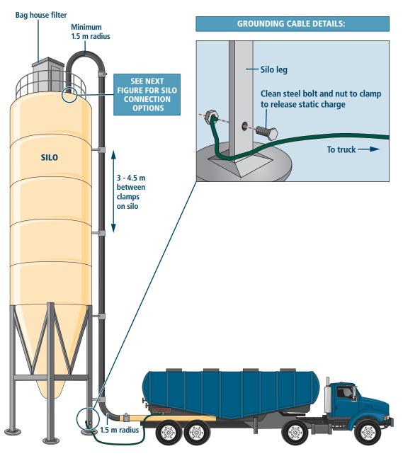
**FIGURE 7.4A.** Recommendations for silo for storage of bulk densified silica fume. Also note grounding recommendations for unloading. See Figure 7.4B for options for connecting the rubber hose to the top of the silo.
