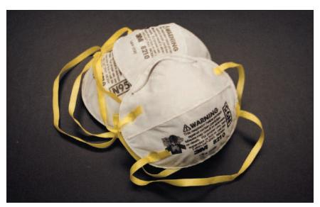
**FIGURE 9.1A.** Dust mask meeting the requirements of 29 CFR 1910.134 and CSA Z94.4-M1982. This mask is recommended for use when working with dry silica fume before it is mixed into concrete in an open, outdoor location. Note that the selection of a mask or respirator must be made on the basis of exposure and environmental conditions. See the following web site for guidance on selecting an appropriate mask: http://www.cdc.gov/niosh/userguide.html.
