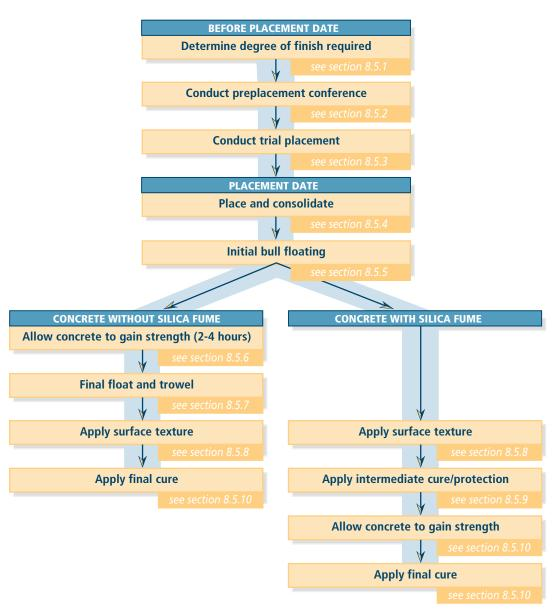
FIGURE 8.13. Finishing steps for concrete flatwork with and without silica fume. The steps are described in the text section noted.
