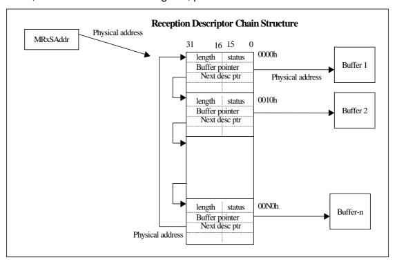
RX Descriptor and buffer must be double word aligned.
