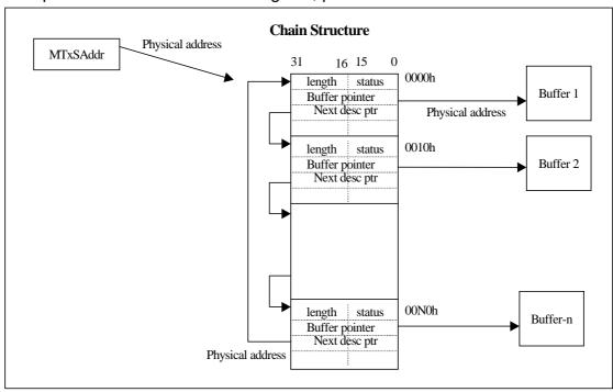
Descriptor must be double word aligned. TX buffer can be at any byte address. MTxSAddr, Buffer\_pointer, Next\_desc\_ptr must be the physical address.
