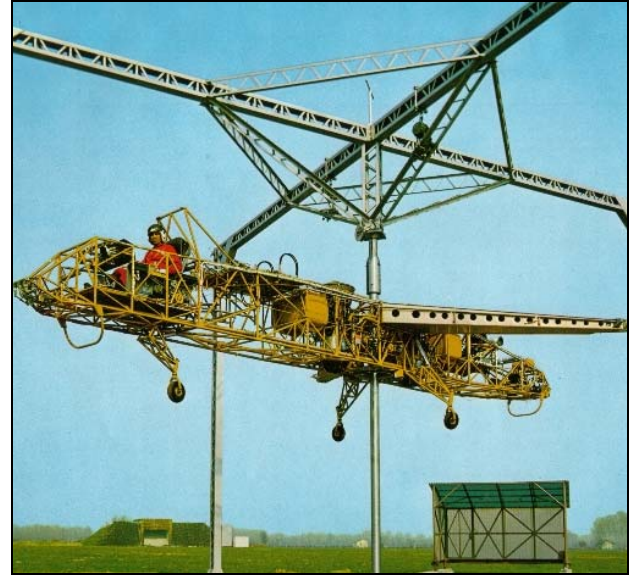
Figure 11. Fiat G.95 test rig in Turin, Italy. [16]
