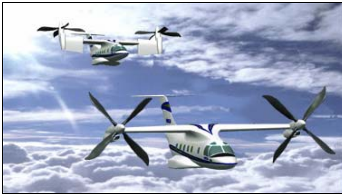
Figure 37. Rendering of ERICA tiltrotor in transition.
