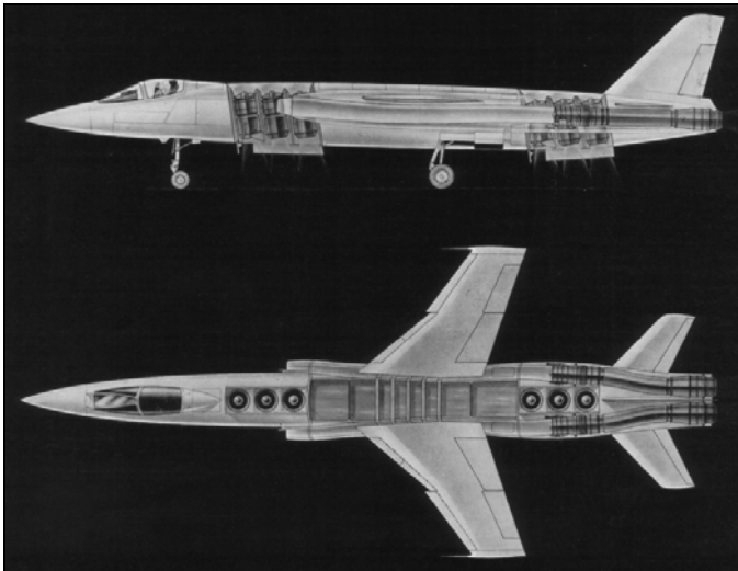
Figure 3. Fiat G.95/6 propulsion system layout.
