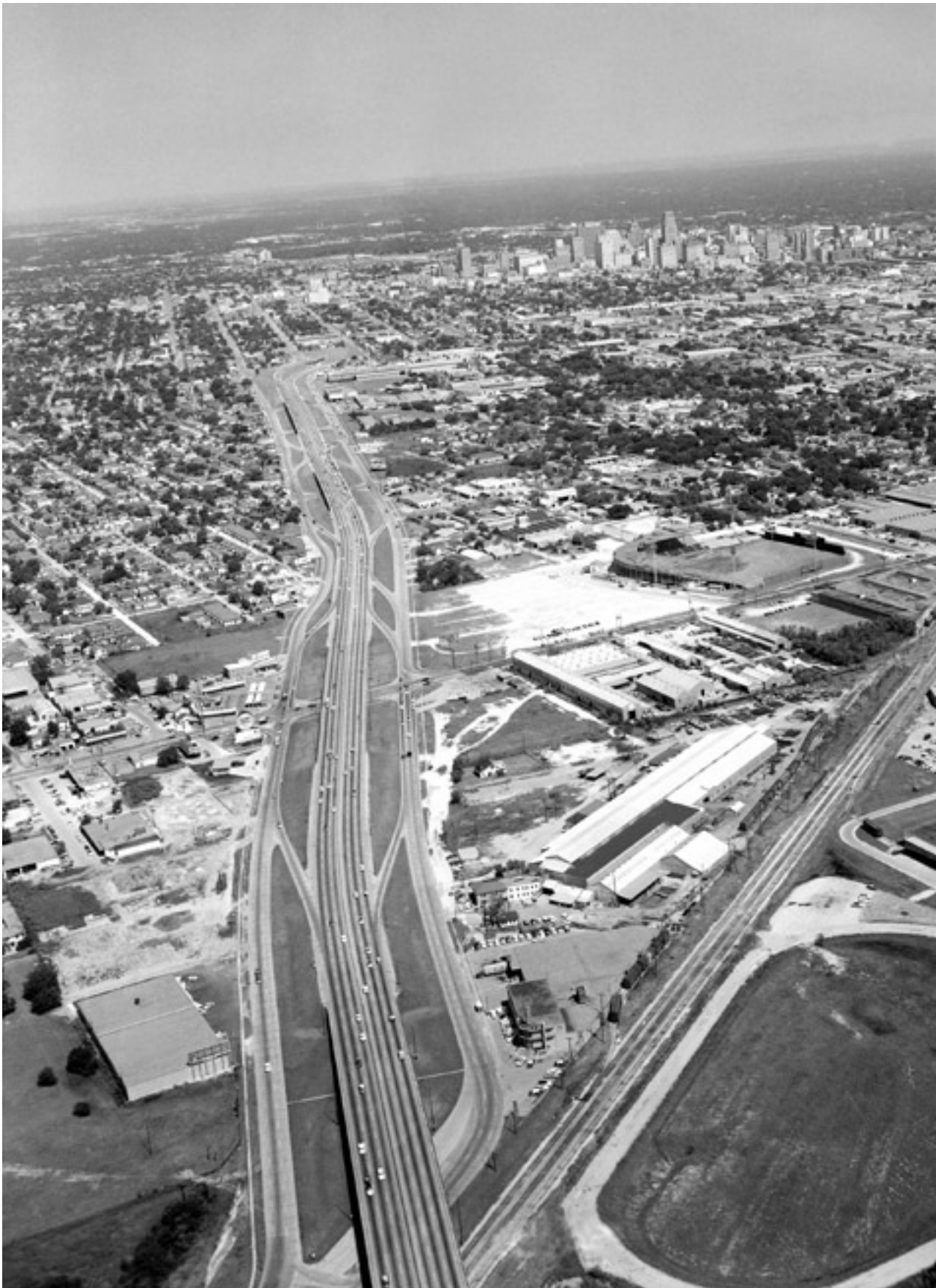
The prototypical Houston freeway: This 1950s aerial view looking toward downtown illustrates one of the key features that would define urban freeways in Texas, and especially in Houston: the frontage road. Although freeways with frontage roads had previously been built in other cities, those instances were typically special cases, often the result of previously existing roads. On the Gulf Freeway, frontage roads were part of a policy and design philosophy that frontage roads should be built whenever possible. This view shows that the original frontage roads did not extend over the railroad tracks, consistent with the policy of serving local traffic, not through traffic, with frontage roads. (Photo: TxDOT)
