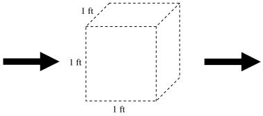
Figure 1 – One Cubic Feet of Volume
