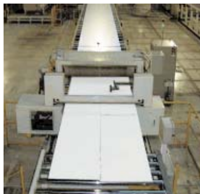
NF Board production line
