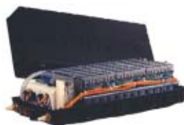
Exhibit 5.1 Cobasys Ni-MH HEV battery pack
