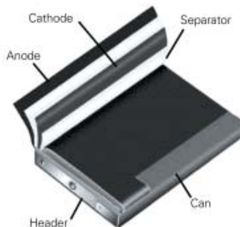
Exhibit 4.8 (a) Sony prismatic cells; (b) cross-section of a prismatic cell
