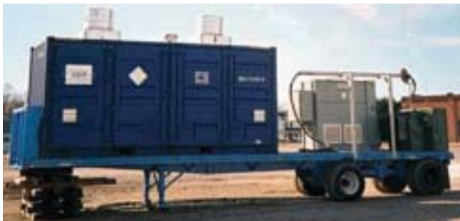
Exhibit 7.14 500 kWh transportable Zn-Br BESS (source: ESA/ZBB)
