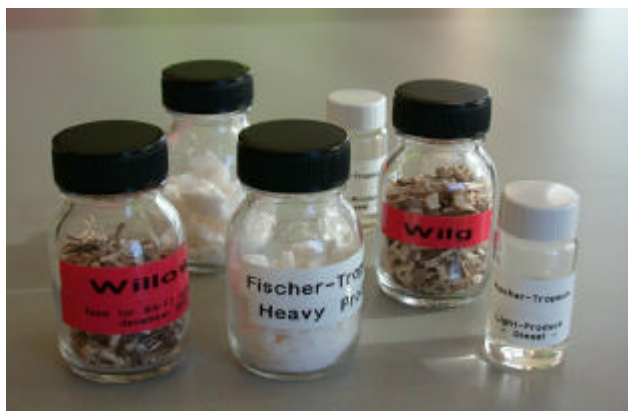
Figure 7. Pictures of the willow used for the integrated test, Fischer-Tropsch wax, and the light product (viz. 'green diesel').
