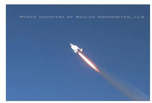
SpaceShipOne. Behind the controls of SpaceShipOne's second successful powered flight was pilot and future astronaut, Peter Siebold. The engine burned for 40 seconds and reached a speed of approximately Mach 1.6, making it the first privately built space vehicle to accomplish this feat.
