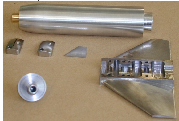
Figure 9: Already manufactured parts of the current LFBB wind tunnel model
