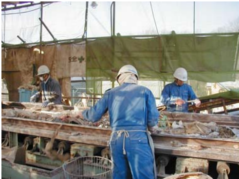
Photo 7 Manual segregation of mixed waste
