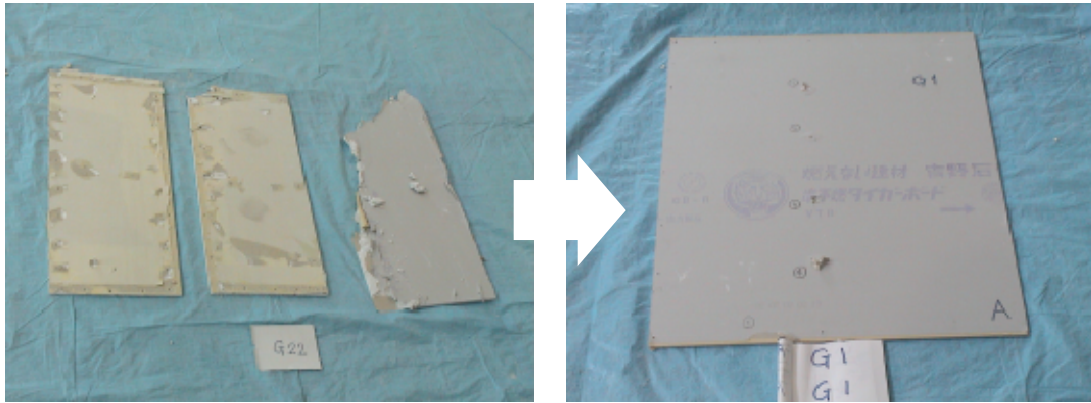
Photo 16 Damage of the gypsum board. Right: “Improved”. The gypsum board generated from the improved test house is less damaged than that of the gypsum board generated from the benchmark test house.
