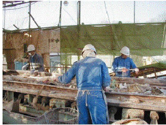
Photo11 Line separation process of the mixed waste.
