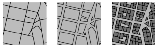
Figure 10: Left: Resulting street map. Middle: Blocks created by scaling from street crossings. Right: The generated lots. Allotments too small or without street access are removed.
