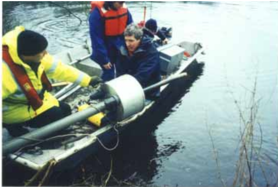
Plate 2 Makereth Sediment Sampling Equipment
