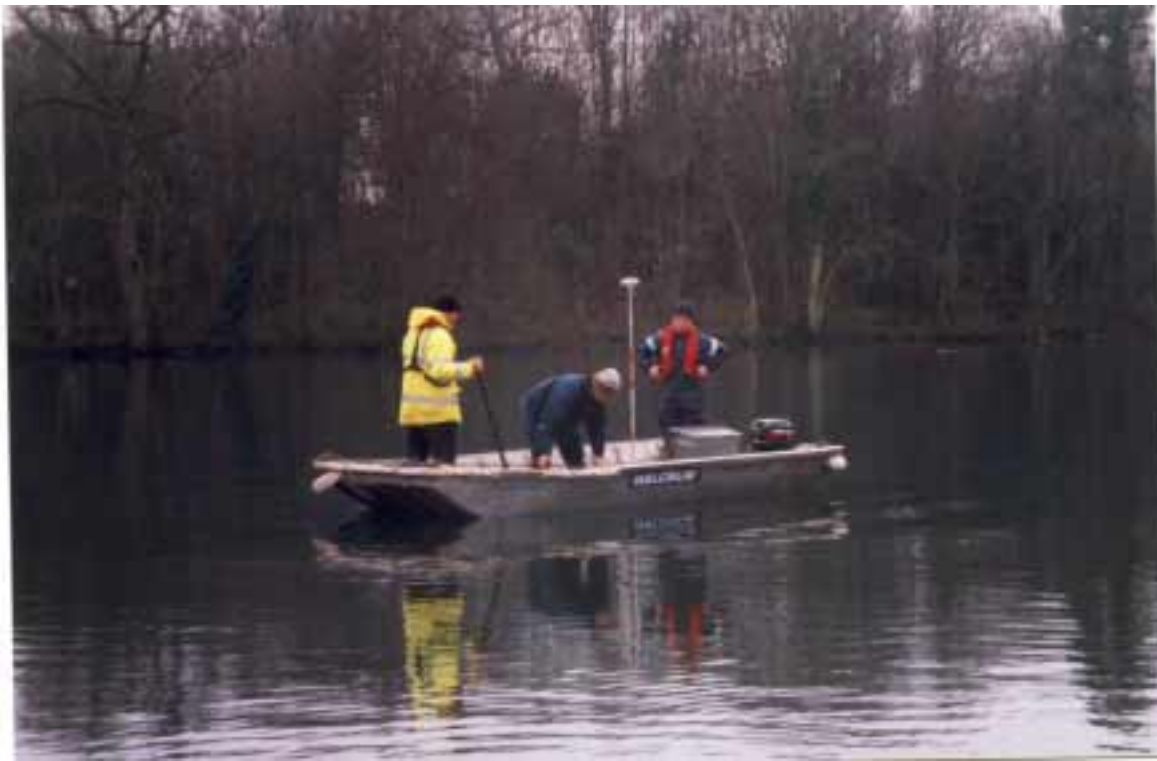
Plate 1 In situ Vane test and Sediment Sampling at Reservoir A
