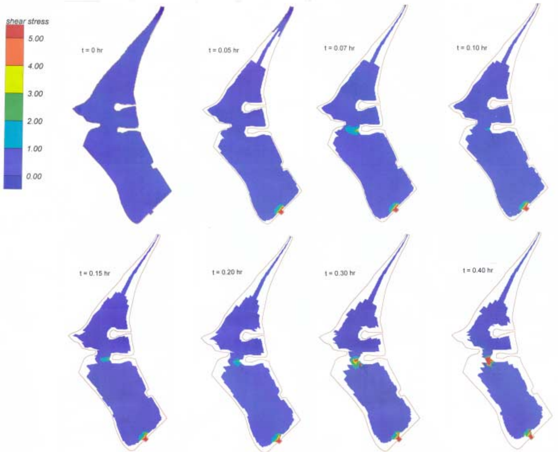
Figure 6.7 Reservoir A Dambreak - Development of Bed Shear Stress (N/m 2 ) with 'Sunny Day' Inflow Conditions
