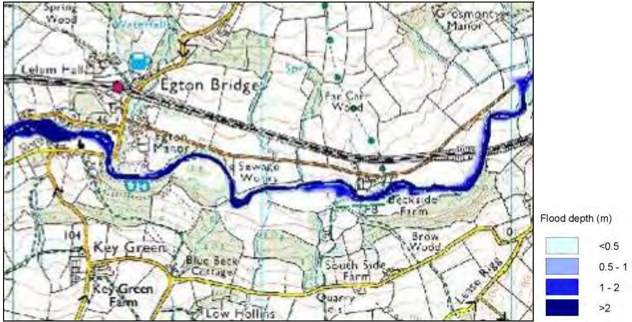
Figure 3.5 – Flood depth at Egton Bridge (1 per cent annual occurrence assuming no defences)
