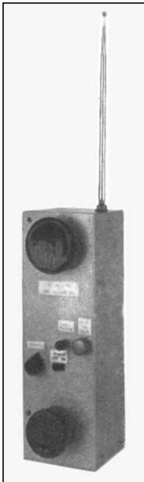
Figure 7—Photo accompanying an article on the construction of a 220 MHz handheld radio for civil defense use.
