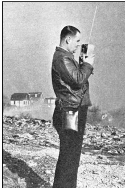
Figure 1—This wartime photo shows a ham operating a 2½ meter handheld transceiver used for emergency communications.
