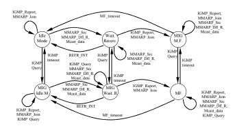
Fig. 6. State diagram illustrating the operation of the MMARP protocol
