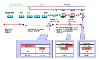
Fig. 2. The proposed MIND architecture with its three constituent parts: the core network, the access network and the ad hoc extension.
