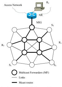
Fig. 5. Example of a MMARP distribution mesh between senders (S) and receivers (R).
