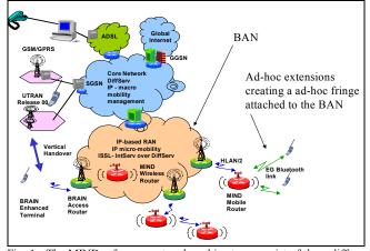
Fig. 1. The MIND reference network architecture consist of three different parts: the core network, the access network and the ad hoc network extension.
