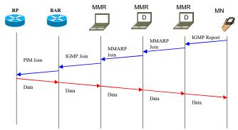
Fig. 3. Example of interaction between the MIND multicast protocols in order to receive a multicast flow
