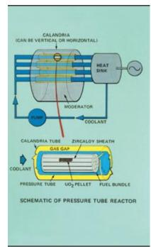
All nuclear reactors operate on the same basic principle, although there are different kinds of nuclear reactors in use throughout the world. A nuclear reactor creates heat by splitting uranium atoms. This "fission" of uranium atoms is called a "nuclear reaction."
