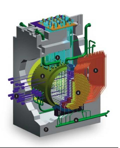
In a closed circuit, the heavy water coolant is pumped through the tubes containing the fuel bundles to pick up heat generated from the nuclear reaction, then to steam generators to produce steam from ordinary water and back to the reactor. The steam is piped outside the reactor containment building to conventional turbines and generators that produce electricity. In this way, the nuclear reactor is separate from the equipment used to produce electricity.
