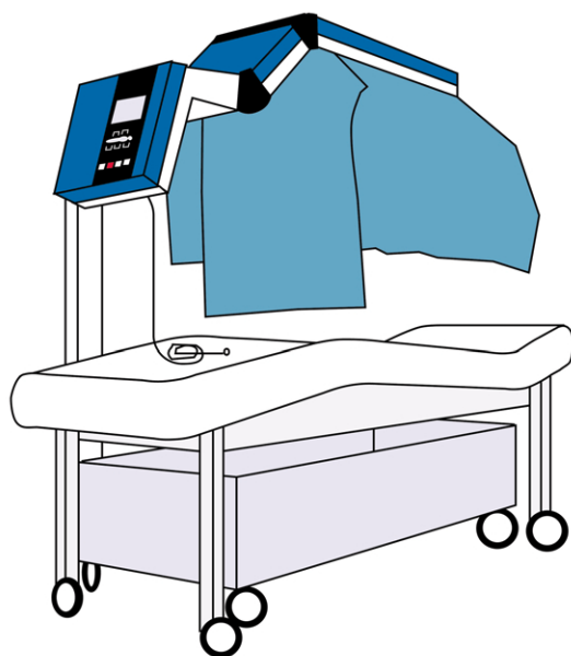
Figure 7. Schematic drawing of the Iratherm system for whole-body hyperthermia. Water-filtered infrared radiators emit their energy from top and bottom. Thermal isolation is ensured by various transport foils. After a systemic temperature of 41.8–42.0°C has been achieved, power is reduced and a steady state is adjusted.
