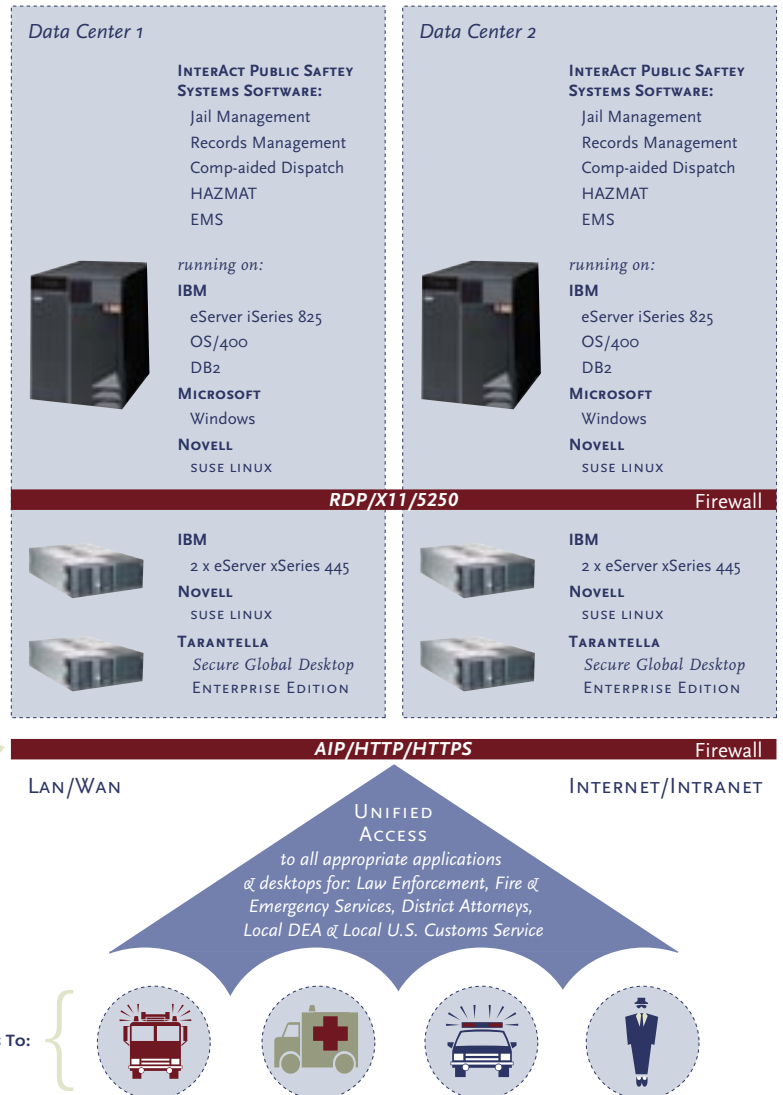
Figure 2: Tri-County inventory using products from InterAct, IBM, Novell, Tarantella and system integration from BCI.
