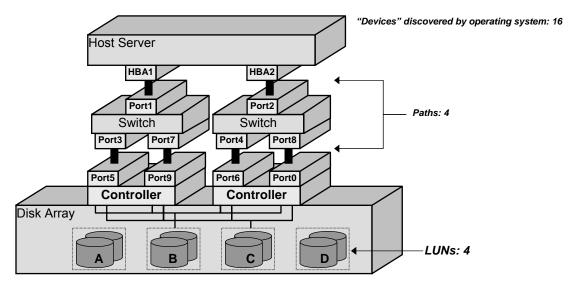
Figure 6: Multi-Port Controllers Connected to Redundant Fabrics
