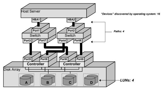
Figure 7: Multi-Port Controllers Cross-Connected to Redundant Fabrics
