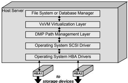
*Figure 8: Generic Model of the UNIX Storage I/O Software Stack*
