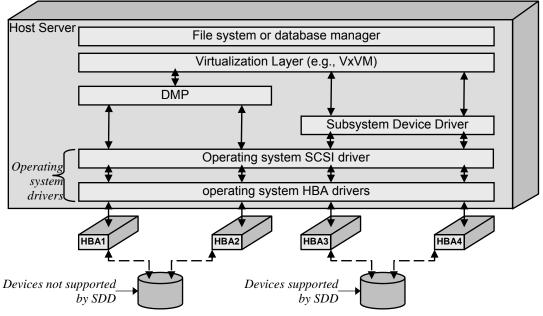
Figure 17: DMP and IBM's Subsystem Device Driver
