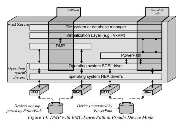
PowerPath is non-suppressing; it leaves operating system nodes for the devices it controls visible in the device tree. DMP does not recognize PowerPath pseudo-devices, but it does recognize sub-paths to devices that PowerPath controls, and will create metanodes and attempt to control them (center shaded area in Figure 14), unless it is prevented from doing so.
