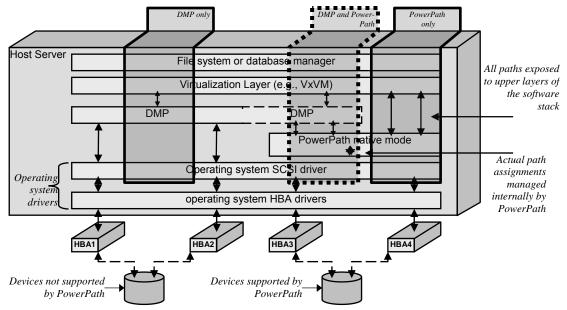
Figure 15: DMP with EMC PowerPath in Native Mode
