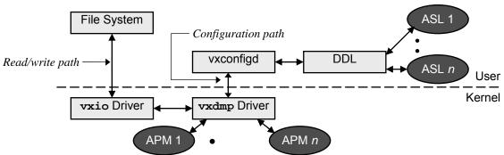
Figure 12: The DMP Device Discovery Layer (DDL) Architecture
