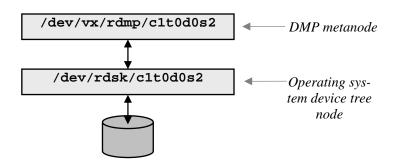
*Figure 9: VxVM Subtree for a Single-Path Device (Solaris)*
