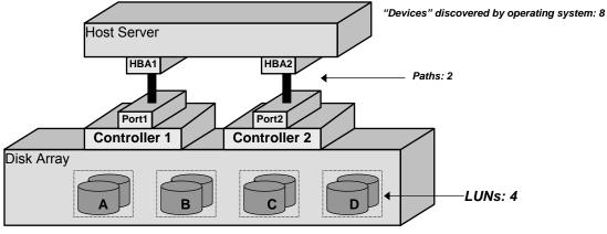
Figure 3: Directly Attached LUNs<sup>5</sup>
