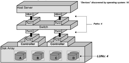
Figure 4: I/O Paths Through a Non-Redundant Storage Network
