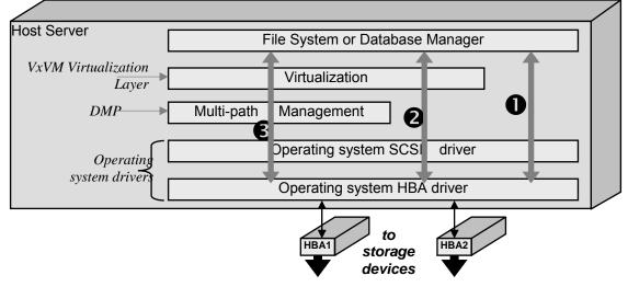
Figure 13: Functions Performed at Different Layers of the UNIX I/O Software Stack
