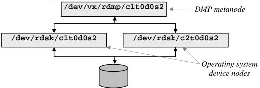
Figure 10: VxVM Subtree for a Dual-Path Device (Solaris)
