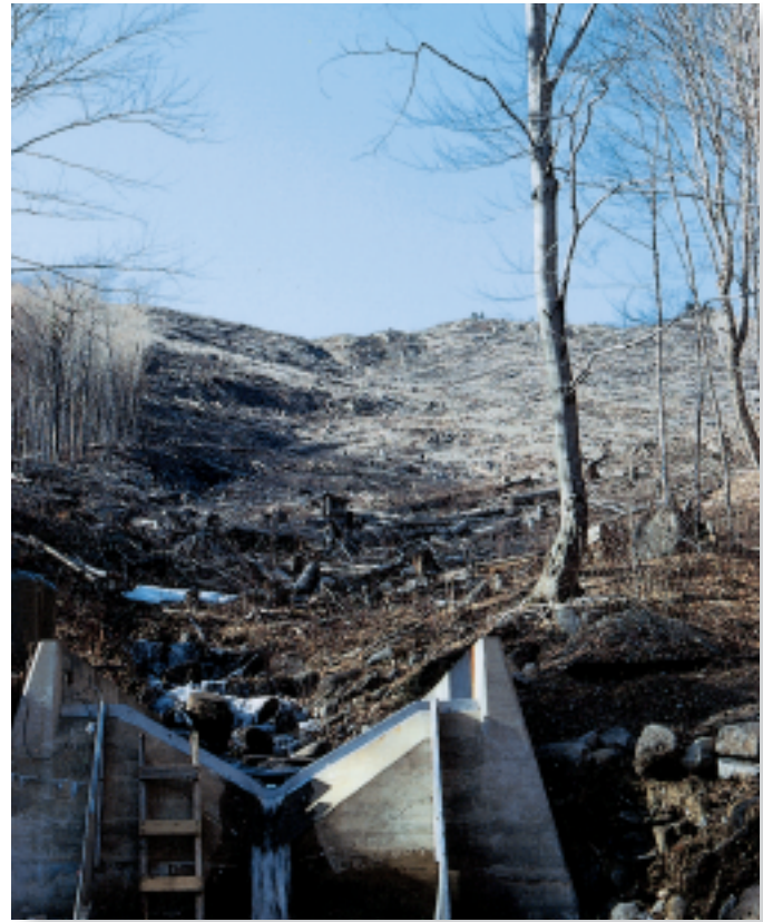
31-5 Hubbard Brook weir Water from each of six experimental ecosystems in the Hubbard Brook Experimental Forest in New Hampshire was channeled through weirs, built where the water leaves the watershed. The water was then analyzed for chemical elements. The trees and shrubs in the watershed behind the weir shown here have been cut down. The experiments showed that deforestation disrupted the tight cycling of nutrients by various living components of the ecosystem and greatly increased the loss of nutrient elements from that system.
