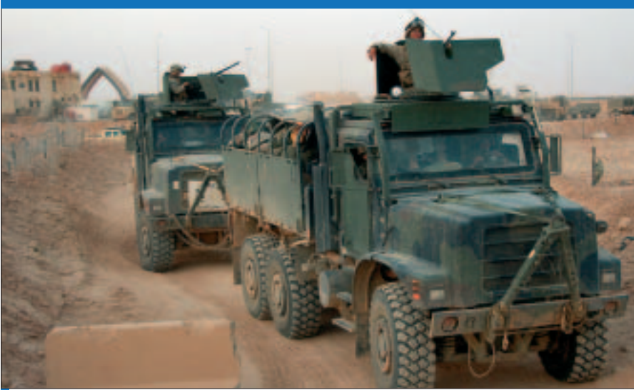
Oshkosh Marine Tactical Vehicle Replacement trucks fitted with armour protection kits are being used on convoy protection and patrol missions in Afghanistan and Iraq. (US Department of Defense)
