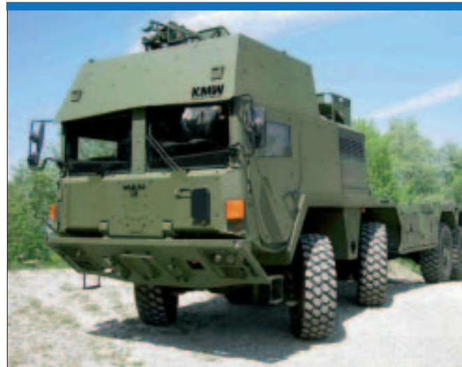
The MAN SX 32.460 8 × 8 logistic truck is fitted with a landmine and ballistic protection package designed by Krauss-Maffei Wegmann. The two manufacturers claim the system offers a level of protection not exceeded by any other logistics vehicle. Pre-series vehicles began field trials with German peacekeepers in Kosovo in 2004. (KMW)
