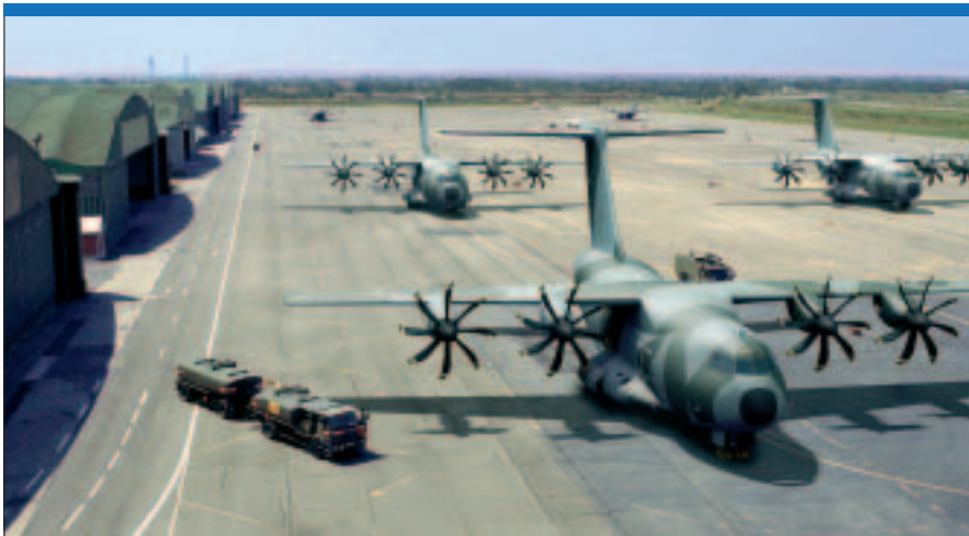
The Airbus Military A400M has gone through a small number of design changes that include the repositioning of the refuelling probe to the port side, and the 'handing' of the propellers. (Airbus Military).
