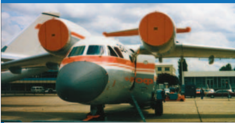
The Antonov An-72/74 appears to have followed the Boeing YC-14 in the use of 'upper surface blowing'. The high engine mounting also reduces foreign object ingestion. (Armada/RB).
