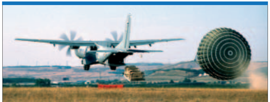
Demonstrating its capability in a low-altitude parachute extraction mission, the Eads-Casa C-295, first flown in 1998, is truly a modern aircraft. It is a stretched derivative of the CN-235 and is adopted by Brazil, Jordan, Poland and Spain. (Eads-Casa).
