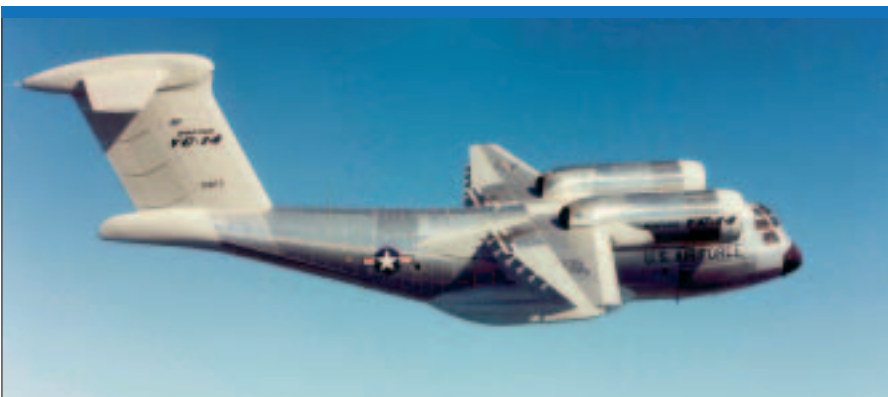
In the mid-1970s the US Air Force planned to replace the C-130 with a jet-powered short-take-off and landing transport. This Boeing YC-14 investigated 'upper surface blowing' to vector thrust. (Boeing).
