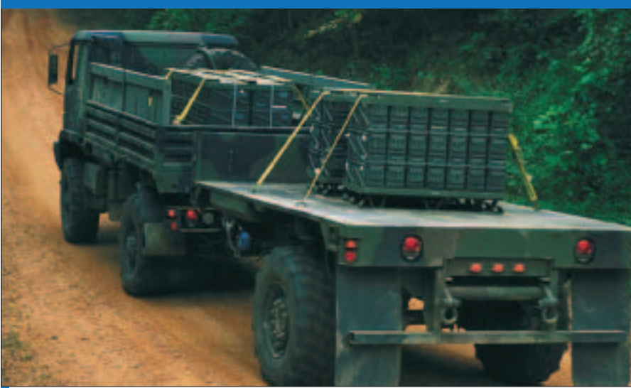
Stewart & Stevenson has produced more than 29,000 examples of the Family of Medium Tactical Vehicle for the US Army with thousands of vehicles still on order. A five-tonne FMTV cargo truck can tow a five-tonne trailer. (Stewart & Stevenson)
