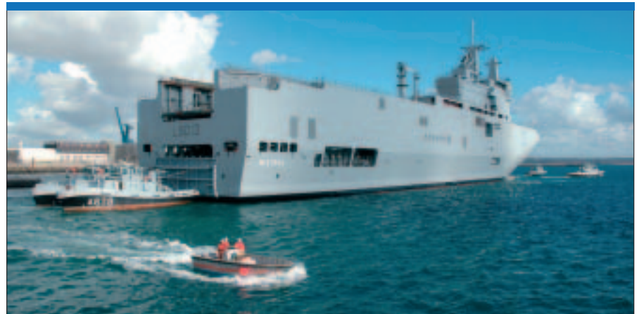
This view of the Mistral clearly shows the wet deck entrance. (DCN International)
