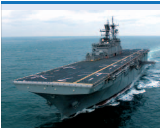
Helicopter carriers such as the HMS Ocean are the spearhead of modern amphibious operations. She can carry 830 troops and deliver them deep inside hostile territory through a dozen medium size helicopters while vehicles and supplies can be brought in by landing craft. (BAE Systems)
