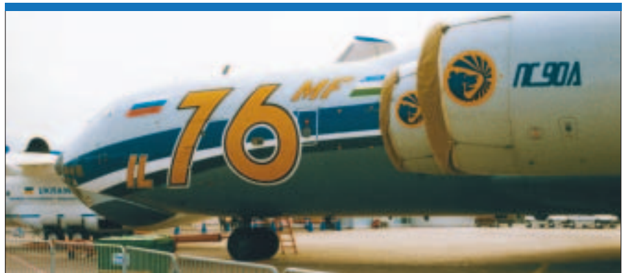
The Ilyushin Il-76MF combines re-engining, as in the case of the civil Il-76TD-90VD with Perm PS-90A turbofans, and fuselage plugs, giving a 6.6-metre stretch. (Armada/RB).
