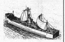
mainsail and jury masts carried the after sail. Under this rig the ship made seven knots for many hours until her engines could be repaired enough to go ahead at two-thirds speed. LSM 229 eventually arrived—late but safe—at Guam.—C. C. Hughes, BMC, USN.
