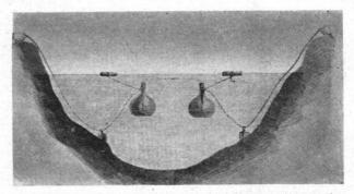
THIS TORPEDO could sink a vessel in ten minutes by brushing one of its floats against the ship's hull.
