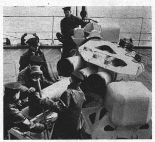
BRITISH new anti-submarine weapon, Squid, is loaded on quarterdeck of the new destroyer, HMS Daring.
