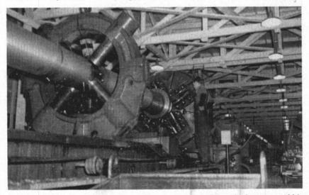
MACHINIST trues up the bearing surfaces of a huge drive shaft as part of his duties at a naval shipyard—one of many operating to keep Navy ships fit.
