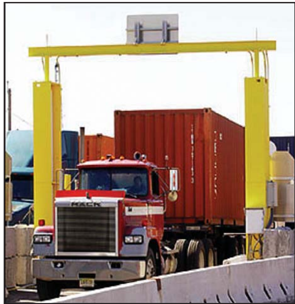
Figure 9: A truck passes through a radiation portal at a port in Newark, NJ. These portals collect data that is used to determine whether the vehicle is carrying illegal RN materials. 14
