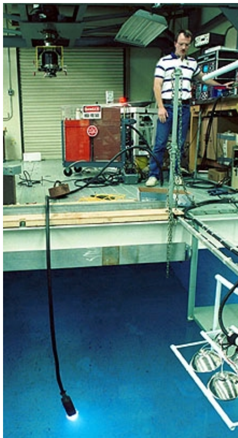
Figure 5.5. Plasma Sound Source electrode in water 341
