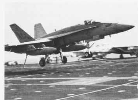
A VFA-305 F/A-18 Hornet catches the wire on board Enterprise .
