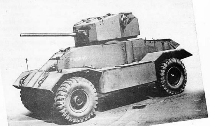
With slightly different hull—the A.E.C. Armoured Car Mark II.
